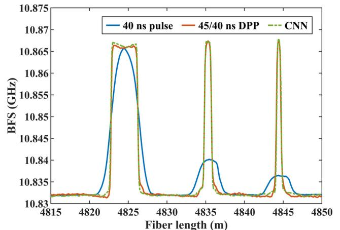
Fig. 5. 40 ns pump pulse measurement results, the CNN output results and 45/40 ns DPP measurement results in the experiment
