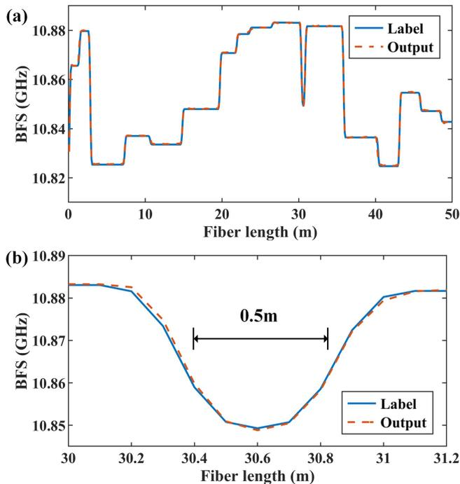
Fig. 3. (a) The comparison between BFS label and CNN output results, (b) The BFS label and CNN output results at 0.5 m changing region.
