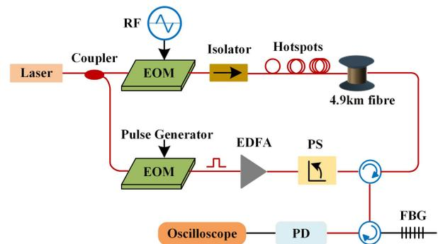
Fig. 4. Experimental setup of the BOTDA system. RF: radio frequency, EOM: electro-optic modulator, PS: polarization switch, EDFA: erbium-doped fiber amplifier, FBG: fiber Bragg grating, PD: photodetector.
