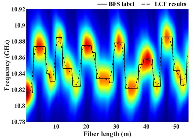
Fig. 2. The simulated BGS and the corresponding BFS label of a set of the training data.
