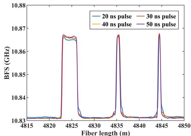
Fig. 7. BFSs retrieved by CNNs from different pump pulse widths between 20-50 ns
