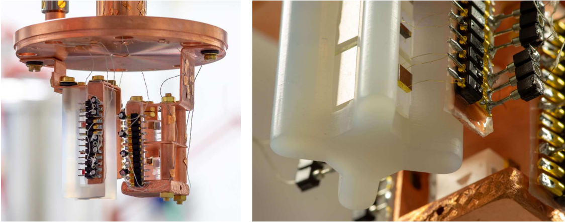
Fig. 3. Picture of the setup containing the two towers wired and installed below the cold plate through S-shaped copper strips ( left ). Detail of the acrylic holder ( right ). It is possible to see the NTDs glued on the crystals and their gold wire link to the Cu strips of the pins. These strips are not thermally coupled to the crystals. Only two channels for acrylic holder and one reference channel in the copper were used for this paper purposes
