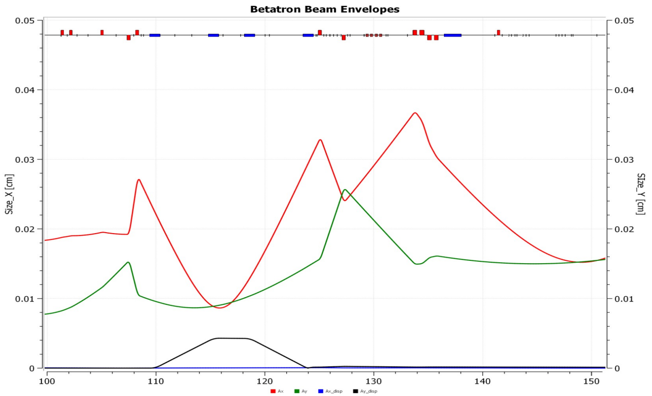
Figure 10. Beam envelopes of interim layout optimized for spot size at pivot (right edge of plot)
