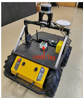
Fig. 4. The experimental setup of a Pozyx UWB Developer Tag mounted on a Clearpath Husky mobile robot.
