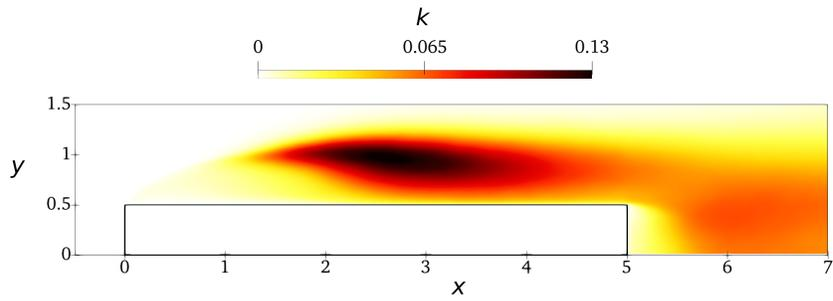
Figure 6: Map of the turbulent kinetic energy for the sharp configuration.
