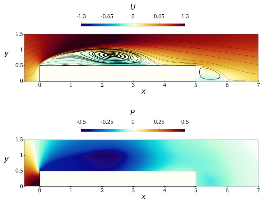
Figure 2: Mean flow. Top: streamlines and color contour for the mean streamwise velocity component  $U$ . Bottom: mean pressure  $P$ .
