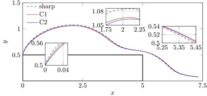
Figure 4: Mean streamline passing through the point  $(x, y) = (0, 0.5001)$ , for the sharp and rounded configurations. The zoomed insets highlight three regions close to the LE, close to the top of the primary recirculation, and in the near wake.
