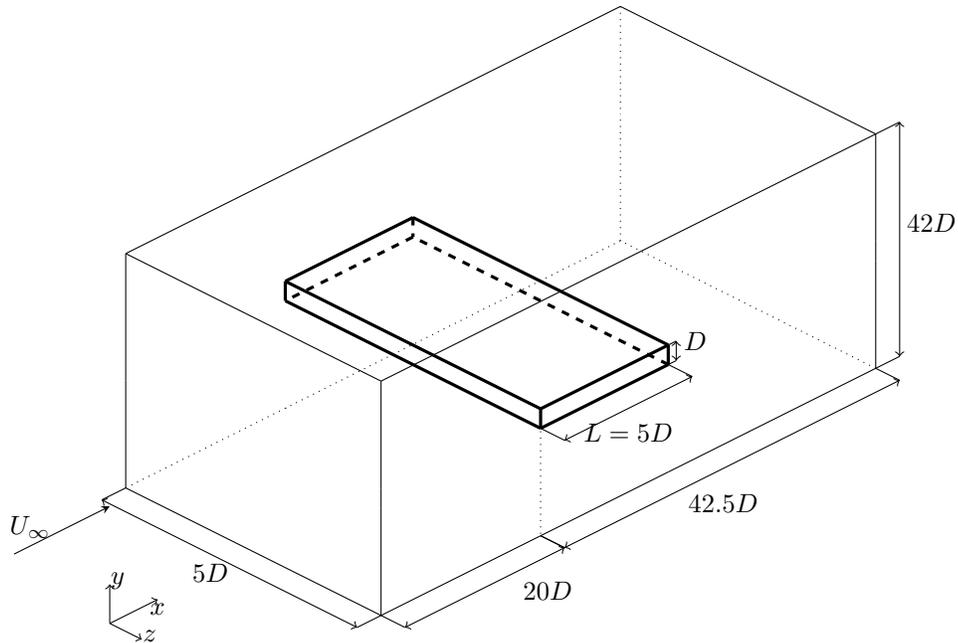
Figure 1: Sketch of the computational domain for the BARC flow, with the reference system.
