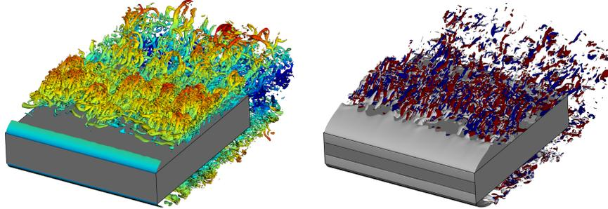
Figure 3: Vortical structures in an instantaneous snapshot. Left: isosurface  $\lambda_2 = -10$  coloured with  $|y|$ ; the blue-to-red colourmap goes from  $|y| = 0.5$  to  $|y| = 1.75$ . Right: isosurfaces of  $\omega_x = 10$  (red),  $\omega_x = -10$  (blue) and  $|\omega_z| = 17$  (grey).
