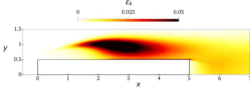
Figure 10: Map of the dissipation rate of the turbulent kinetic energy
