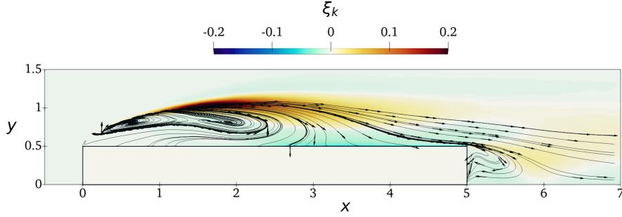
Figure 12: Field lines of the flux vector  $\psi$  and colormap of the source  $\xi_k = P_k - \epsilon_k$  for the reference sharp configuration. The arrows are tangent to the flux vector  $\psi$  and provide directional information.
