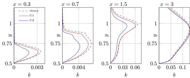
Figure 7: Vertical profiles of the turbulent kinetic energy  $k$  at four different stations over the cylinder side, i.e.  $x = 0.3, 0.7, 1.5, 3$ .
