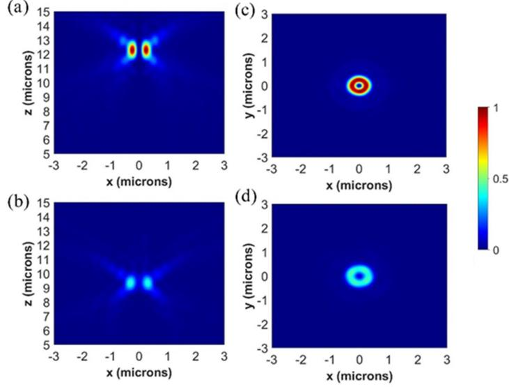
Fig.3 (a) and (b) are simulated electrical field intensity patterns in the  $x-z$  plane generated by Metalens1 under illumination of an LCP and RCP incident beam, respectively. (c) and (d) are simulated intensity distributions of the converged vortex beams in different focal planes ( $z = 12.3\mu\text{m}$  or  $9.3\mu\text{m}$ ) for an LCP and RCP incident beam, respectively.
