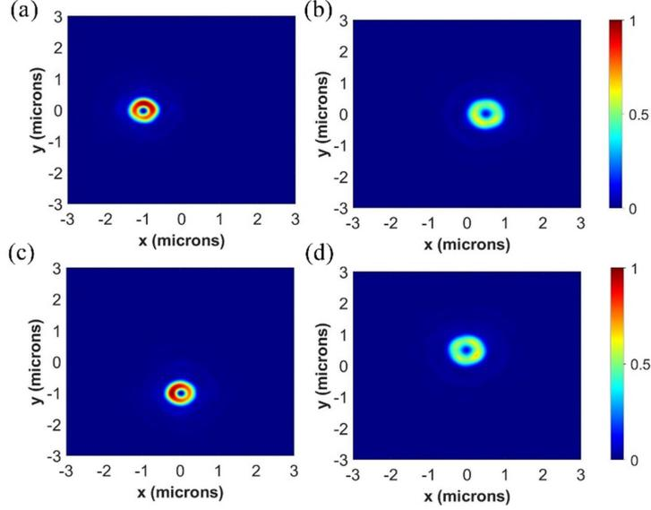
Fig.4 (a) and (b) are simulated intensity distributions of the focused vortex beams generated by Metalens 2 with different  $x$ -direction displacements in the same focal plane ( $z = 9.3\mu\text{m}$ ) for LCP and RCP incident beams, respectively. (c) and (d) are simulated intensity distributions of the focused vortex beams generated by Metalens 3 with different  $y$ -direction displacements in the same focal plane ( $z = 9.3\mu\text{m}$ ) for LCP and RCP incident beams, respectively.
