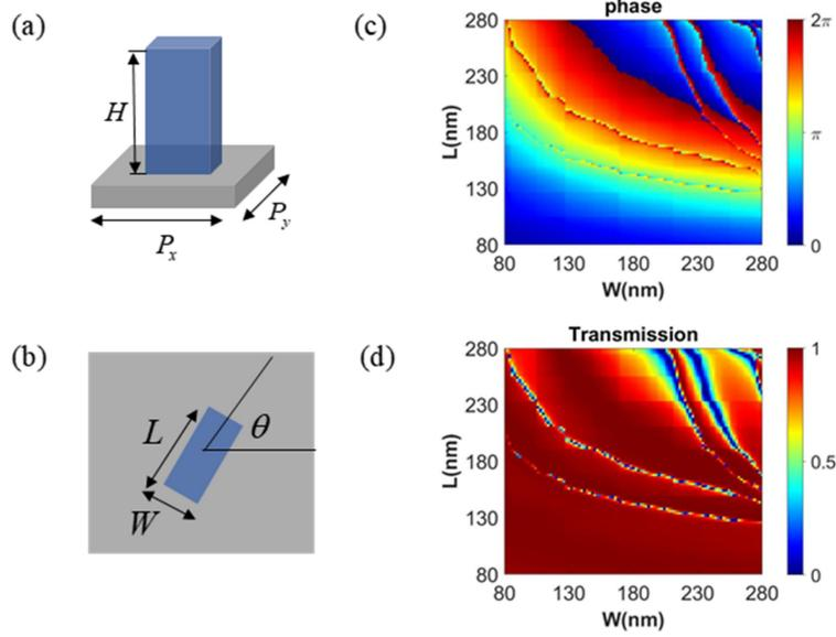
Fig.2 (a) and (b) are side view and vertical view of typical unit cell of the spin-dependent metalens with the period ( $P_x$  and  $P_y$ ), height ( $H$ ), varying cross sizes ( $L$  and  $W$ ), and different rotation angles ( $\theta$ ). (c) and (d) are simulated propagation phase and transmission distributions for an XLP incident beam, respectively.
