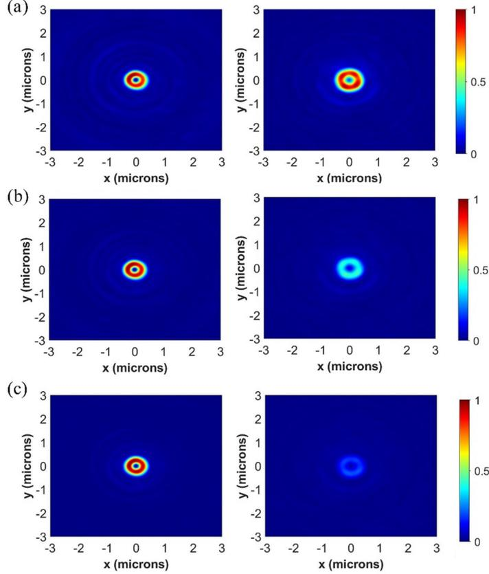
Fig.5 The intensity distributions of the focused vortex beams generated by Metalens 1 in different focal planes (left:  $z=12.3\mu\text{m}$ ; right:  $z=9.3\mu\text{m}$ ) when (a) ellipticity of the incident beam is  $1/5$ , (b) ellipticity of the incident beam is  $0$ , and (c) ellipticity of the incident beam is  $-1/5$ .
