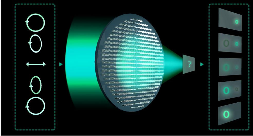
Fig.1 Schematic of the spin-dependent metalens with intensity-adjustable dual-focused vortex beams. The pattern in the left dotted-box represents the polarization state of the monochromatic incident beam; their corresponding monochromatic focused vortex beams are shown in the right dotted-box. Note that the patterns of polarization state and focused vortex beams in these two dotted boxes are in horizontal correspondence.
