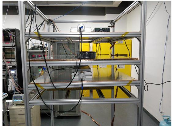
**Figure 10:** Cosmic test system
