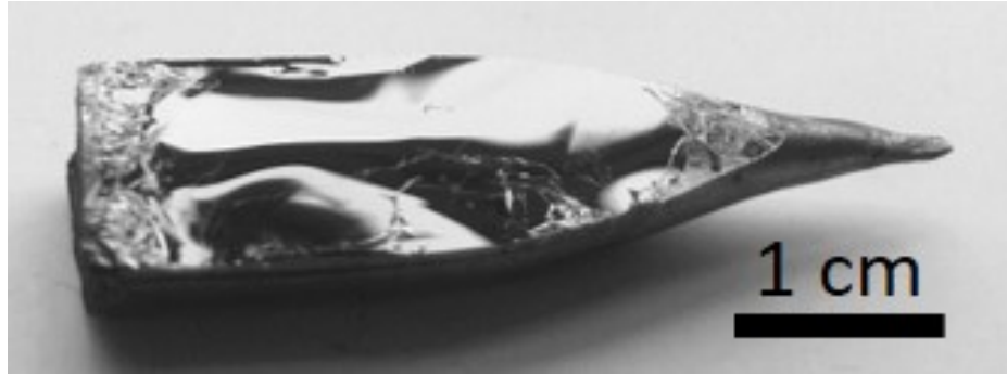
Fig. 6. Photograph of a p-InSe ingot cleaved parallel to the c-plane.
