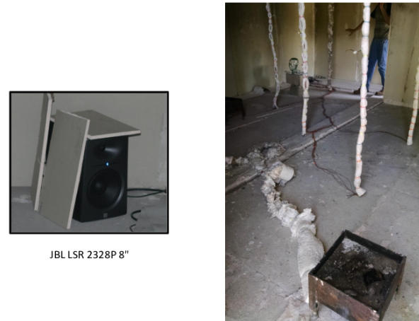
FIG. 3. (Color Online) Photograph of the inside of the burn structure showing the burner, manikin, and speaker used in the HRTF measurement. Several thermocouple trees are visible. The propane line to the sand burner is protected by 2-inch-thick kaowool insulation, and the speaker is protected from the heat using 3/16-inch-thick sheets of gypsum drywall.
