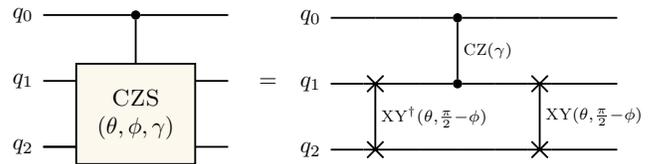
Figure 2. Decomposition of the three-qubit CCZS gate into two-qubit gates. Note that for the case of a linear chain [see Fig. 1(a)], the control qubit  $q_0$  in the CCZS gate is the middle qubit, but the decomposition into two-qubit gates requires  $q_1$  to be the middle qubit, since it has to interact with both  $q_0$  and  $q_2$ .
