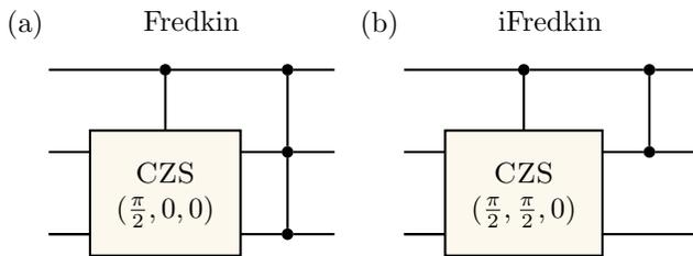
Figure 3. Converting CCZS gates into other three-qubit gates. (a) Constructing a Fredkin gate with a  $CCZS(\pi/2, 0, 0)$  gate and a CZ gate. (b) Constructing an iFredkin gate from a  $CCZS(\pi/2, \pi/2, 0)$  gate and a CZ gate.
