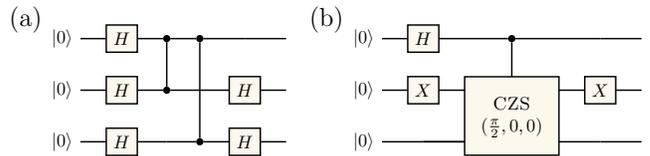
Figure 4. Quantum circuits for generating the three-qubit GHZ state  $(|000\rangle + |111\rangle)/\sqrt{2}$ . (a) A circuit using single-qubit gates and two-qubit CZ gates. (b) A circuit using single-qubit gates and one CCZS gate.
