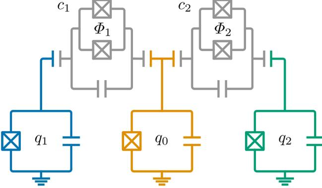
Figure 9. Setup for implementing the CCZS gate with tunable couplers  $c_1$  and  $c_2$  connecting the qubits. The frequency of each coupler  $j$  is tuned by changing the magnetic flux  $\Phi_j$  through the loop formed by the two Josephson junctions.
