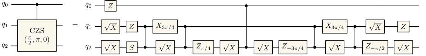
Figure 8. Decomposition of the CCZS( $\pi/2, \pi, 0$ ) gate into single-qubit and CZ gates, obtained using Qiskit [140]. For the single-qubit gates, we use the notation  $S = \sqrt{Z} = Z_{\pi/2}$  and  $\sqrt{X} = X_{\pi/2}$ . Note that this decomposition requires qubit 2 being placed in the middle of the linear chain, since it has to perform CZ gates with both qubit 0 and qubit 1.
