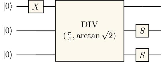
Figure 13. Quantum circuit for generating the three-qubit W state  $(|100\rangle + |010\rangle + |001\rangle)/\sqrt{3}$  using the DIV gate. The phase gate S is  $\sqrt{Z}$ .
