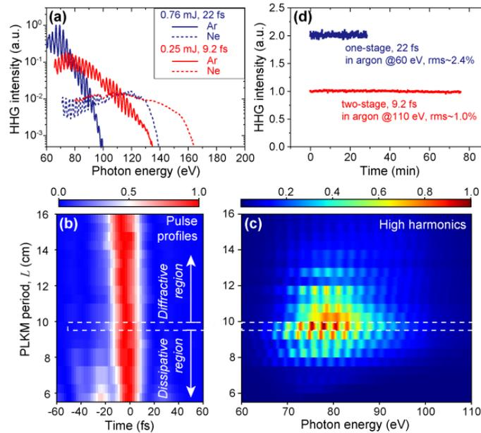
Fig. 5. (a) The HHG spectra driven by compressed pulses in argon and neon. (b) The pulse intensity profiles measured by SHG-FROG under different PLKM periods  $L$  of the second-stage compressor. The optimum condition is determined to be  $L=9.5$  cm. The dissipative and
