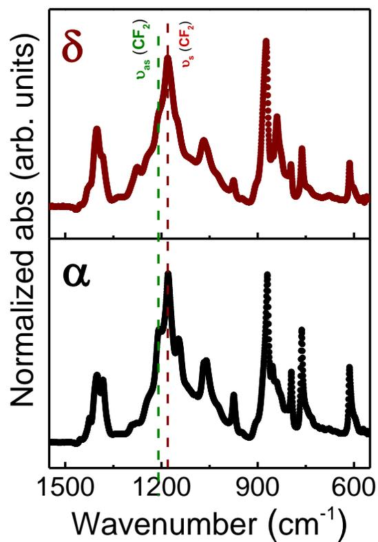
FIG. S3. FT-IR spectra of PVDF nanoparticles with  $\delta$  and  $\alpha$ -phase. The upper panel (marked as  $\delta$ ) is for as prepared  $\delta$ -PVDF nanoparticles and the lower panel (marked as  $\alpha$ ) is for  $\alpha$ -PVDF, when the phase transformation is attained by thermal treatment at 170°C.
