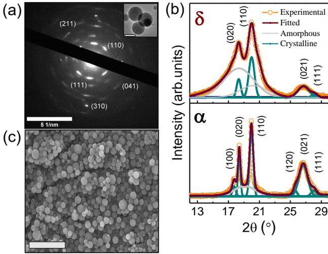
FIG. 1. (a) SAED pattern of  $\delta$ -phase in PVDF nanoparticles. Inset shows the TEM imaging of PVDF nanoparticles (scale bar 200 nm). (b) X-ray diffraction pattern of PVDF nanoparticles in different phases. Experimental observation of  $\delta$ -phase at 30°C (marked as  $\delta$ ) and its conversion to  $\alpha$ -phase at 170°C after temperature treatment (marked as  $\alpha$ ). (c) Morphology of  $\delta$ -PVDF nanoparticles as uniform distribution in SEM (scale bar 5  $\mu\text{m}$ ).
