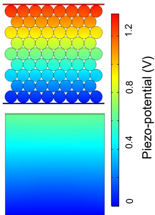
FIG. S6. FEM based theoretical simulation for PVDF nanoparticles and planar film. It shows the relative generated piezo-potential under the application of 100 kPa pressure in both cases.
