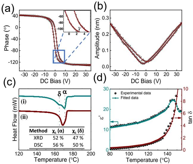
FIG. 2. (a) Phase (b) Amplitude response of  $\delta$ -PVDF nanoparticles in PFM, after applying a DC bias of  $\pm 35$  V. Temperature dependent study of  $\delta$ -PVDF nanoparticles as (c) Heat flow in DSC at  $1^\circ\text{C}/\text{min}$ . followed by (i) first heating (ii) second heating cycle (inset shows the estimated crystallinity from DSC and XRD). (d) Dielectric constant ( $\epsilon'$ ) and loss tangent ( $\tan \delta$ ) of  $\delta$ -PVDF for variable temperature at 1 kHz frequency.
