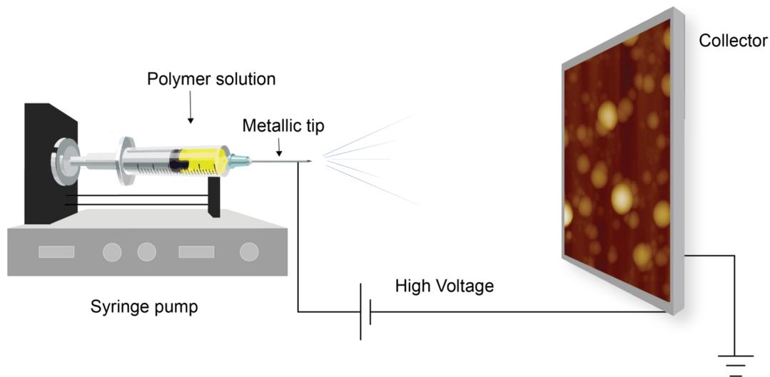
FIG. S2. Schematic of electro spray setup, where a high voltage is applied between metallic tip and collector.
