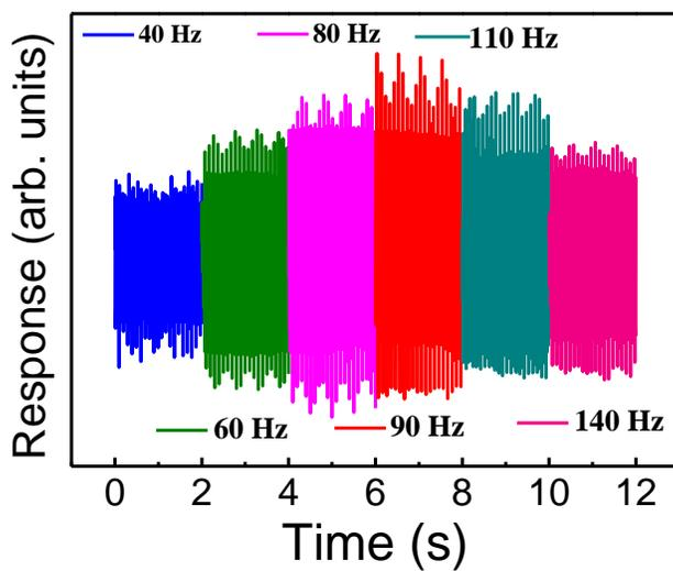
FIG. S7. Acoustic response of NG at various frequencies with acoustic sensitivity of  $\sim 2.75$  V/Pa.
