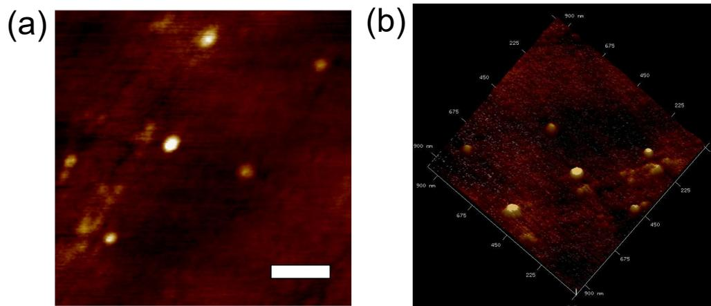
FIG. S4. (a) AFM topography of  $\delta$ -PVDF nanoparticles with (a) 2D and (b) 3D view (scale bar 225 nm).
