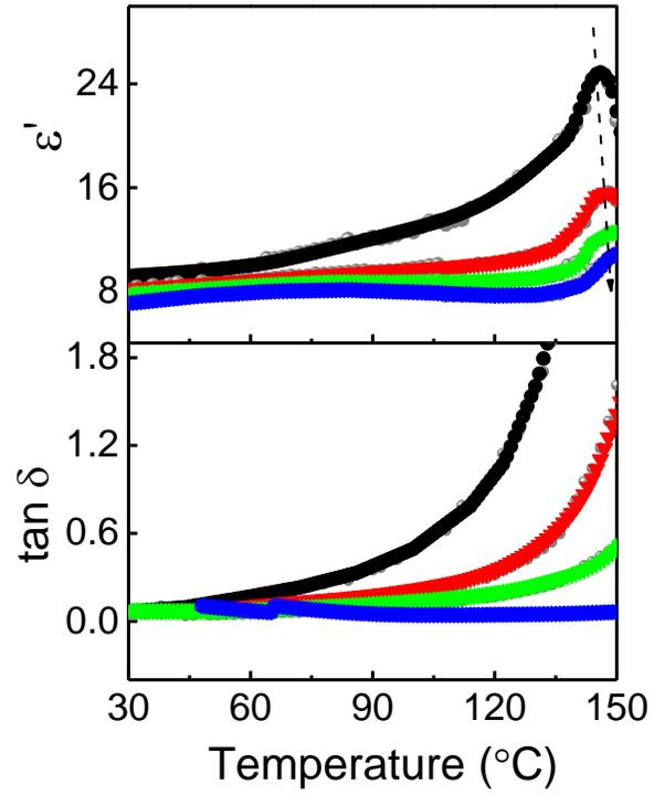
FIG. S5. Dielectric constant ( $\epsilon'$ ) and loss tangent ( $\tan \delta$ ) of  $\delta$ -PVDF nanoparticles with variable temperature range of 30-155°C at certain frequencies, viz., 1, 10, 50 and 500 kHz.
