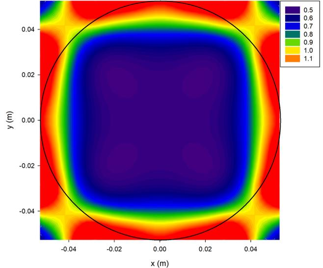
FIG. 9. 2D colour plot of magnetic field in the cross-section at  $z = -113$  mm where the trap minimum (leakage spot) is located. Colour legend provides field in the range 0.5-1.1 T. The black circle corresponds to the trapping cell inner surface at  $r = 53$  mm. Plots are calculated for the 100% of  $I_t$  (0.8 T trap depth).
