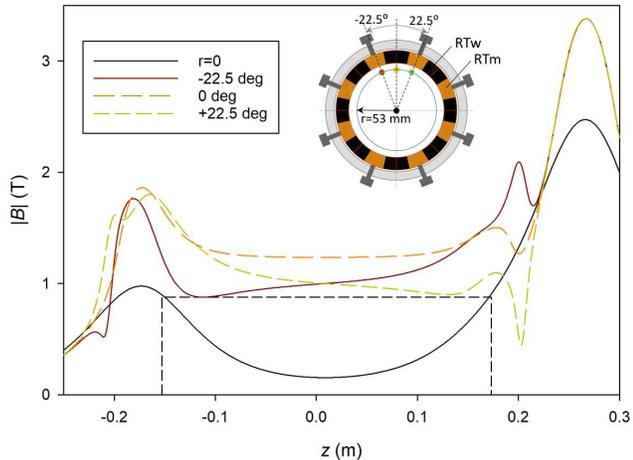
FIG. 8. Magnetic field profiles along several vertical lines parallel to the IPT axis ( $z$ -axis) at the distance of 53 mm from the trap axis. The locations of these lines in the horizontal cross-section are shown in the insert. Vertical dashed lines mark locations of the top and bottom of the trapping cell. Plots are calculated for 100% of  $I_t$  (0.8 T trap depth).
