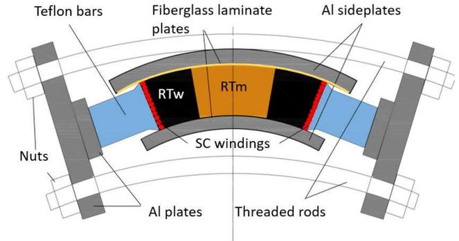
FIG. 5. Pressing tool for linear parts of the race-track coils. RTw - race-track windings; RTm - race-track mandrel; SC windings - superconductive wire windings
