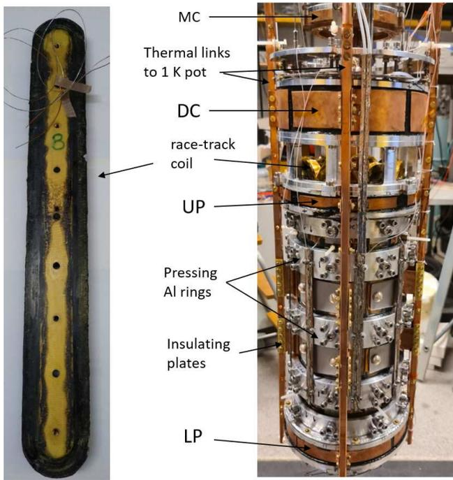
FIG. 7. Photographs of an individual race-track coil just after winding and before finalizing its shape (left) and of the final IPT assembly hanging in the dilution cryostat (right).
