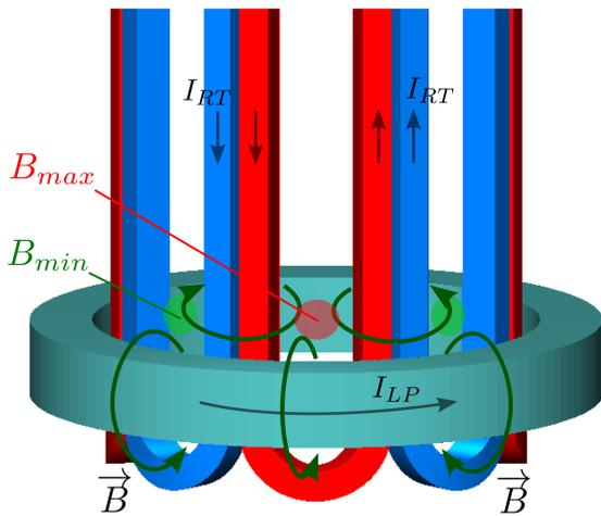
FIG. 4. The configuration of currents and magnetic fields near the edge of the lower pinch in the so-called "leakage spots" of the trap. Due to the alternating direction of the field generated by the octupole segments, for every second race-track, the radial component of this field is subtracted from that of the pinch. These regions near the upper(lower) edge of the lower (upper) pinch define the absolute minimum of the trapping field  $B_{min}^{wall}$  on the wall of the trapping cell.
