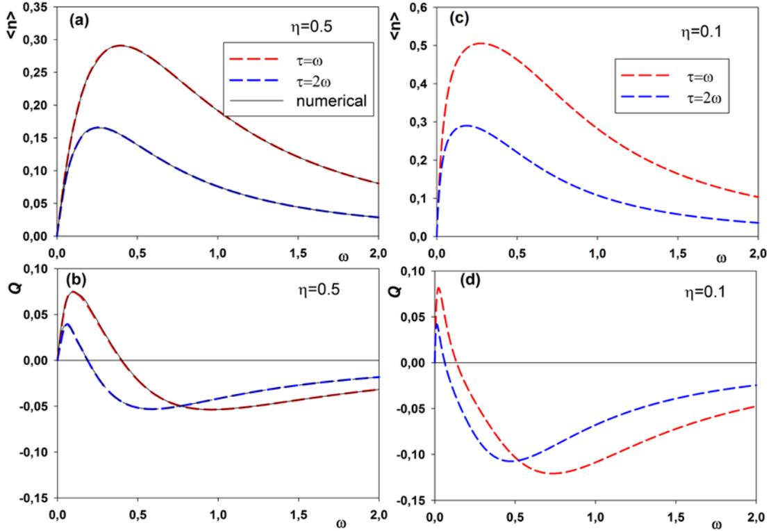
**Figure.** The mean number of photons in the cavity mode (a), (c) and corresponding Mandel  $Q$ -parameter (b), (d) vs  $\omega$ . Solid black lines (a), (b) – numerical calculation of (1); Dashed colour lines – analytical results obtained with the help of (6);  $\tau = \omega$  – dashed red lines,  $\tau = 2\omega$  – dashed blue lines.
