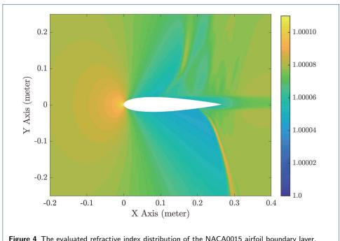
Figure 4 The evaluated refractive index distribution of the NACA0015 airfoil boundary layer.
