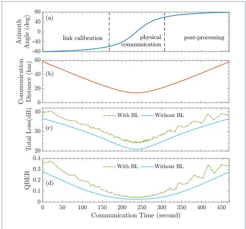
Figure 8 (a) Azimuth angle over the flight time. (b)The communication distance between the aircraft and the ground station. (c) The total loss in the airborne QKD scenario. (d) The estimated QBER over the flight time.
