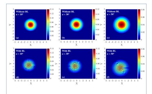
Figure 7 (a)-(c) show the intensity distribution of the beam propagated without the boundary layer effects. (d)-(f) show the intensity distribution of the beam propagated through the boundary layer. Here  $\alpha=10^\circ,30^\circ,50^\circ,$  and the unit of axis is meters.
