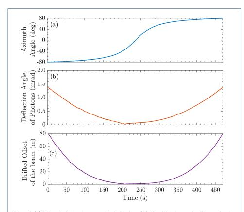
**Figure 6** (a) The azimuth angle  $\alpha$  over the flight time. (b) The deflection angle of transmitted photons. (c) The drifted offset of the beam, which reaches to the ground station.
