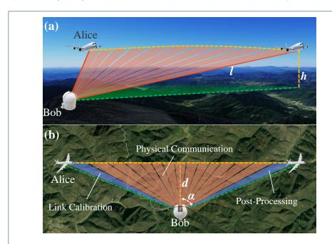
Figure 2 (a) Main view and (b) top view of schematic diagram of downlink airborne QKD. The aircraft (Alice) flies in a certain path obliquely above the receiving ground station (Bob).
