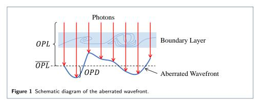
The aero-optical effects are fundamentally caused by the gradient refractive index n due to the variable-density flow field, which is expressed by the Gladstone-Dale equation [46]
