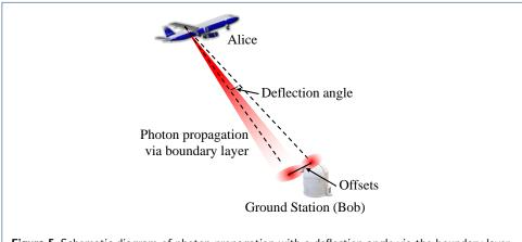
Figure 5 Schematic diagram of photon propagation with a deflection angle via the boundary layer.
