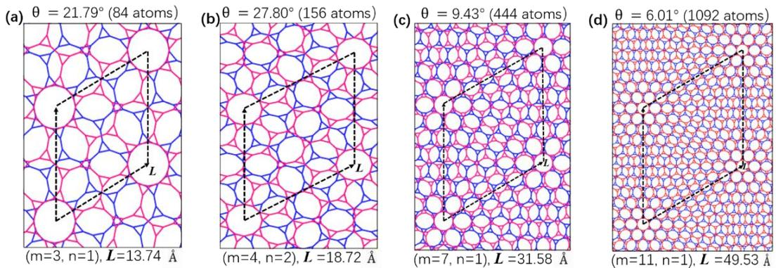
Figure 2. Schematic illustrations of TBKGs with (a)  $\theta = 21.79^\circ$ , (b)  $\theta = 27.80^\circ$ , (c)  $\theta = 9.43^\circ$ , and (d)  $\theta = 6.01^\circ$ . Dashed rhombuses are the primitive cells for the Moiré superlattices. At the bottom of each panel, indices  $(m, n)$  are given, which are related to twisting angle  $\theta$  via Eq. (1).  $L$  is the dimension of the primitive cell.
