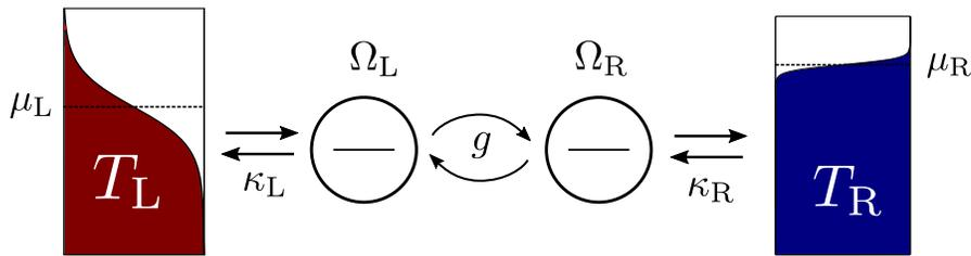
**Figure 4.** System of coupled quantum dots acting as a heat engine. Two quantum dots with on-site energies  $\Omega_L$  and  $\Omega_R$  are coupled to each other with coupling strength  $g$  and to a thermal reservoir of temperatures  $T_L$ ,  $T_R$  and chemical potentials  $\mu_L$ ,  $\mu_R$  (with coupling strength  $\kappa_h$  and  $\kappa_c$ ) respectively.
