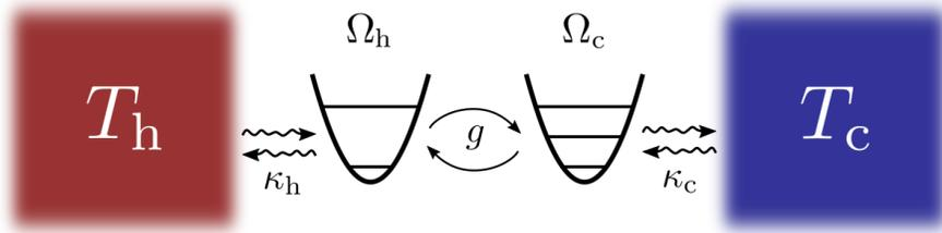
**Figure 1.** System of coupled harmonic oscillators to illustrate the validity of different Markovian master equations. Two harmonic oscillators with frequencies  $\Omega_h$  and  $\Omega_c$  are coupled to each other with coupling strength  $g$  and to a thermal reservoir of temperature  $T_h$  and  $T_c$  (with coupling strength  $\kappa_h$  and  $\kappa_c$ ) respectively.
