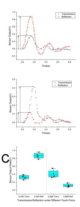
Figure 5: A: Stacked PPG waveforms obtained using the transmission and reflection methods at 0.44N touch force. B: Waveforms obtained at
