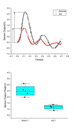
Figure 4: A: Stacked PPG waveforms at different temperatures with a constant touch force of approximately 0.68N. B: Summary of four subjects' results.
