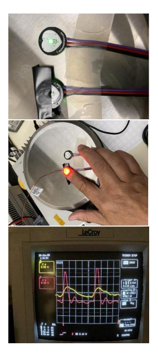
Figure 2: (A) One PPG sensor with the green light exposed and another covered by black tape (B) Red light shines through finger and hits the sensor measuring the transmission signals (C) The measured signals shown on an oscilloscope
