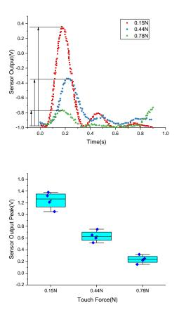
Figure 3: A:Stacked PPG waveforms at different touch force pressures. B: Summary of the sensor responses (peak value) over different subjects.
