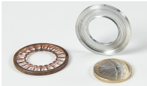
Figure 3. On the left, a copper meta-ring based on the structure shown in Fig. 1, fabricated by additive printing; the aluminum meta-ring on the right is based on the structure shown in Fig. 2 and it is manufactured by traditional machining at a lower cost and with a higher precision [11].
