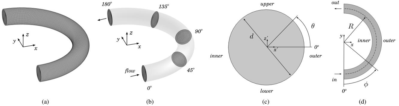
FIG. 1. Curved pipe geometry and orientation. (a) curvature mesh, (b) curved pipe with flow direction and various cross-sections, (c)  $x'z'$  cross-sectional plane viewed from upstream, (d)  $xy$  plane of symmetry.
