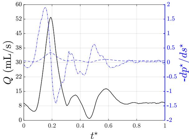
FIG. 3. Flow rate  $Q$  (black solid) “lagging” the straight pipe nondimensional pressure gradient  $-\partial p^*/\partial s^*$  (blue dash dot) at Womersley number  $\alpha = 4.22$ . The pressure gradient from a pulsatile Poiseuille solution (blue dash) required to produce the same flow rate is shown for comparison.
