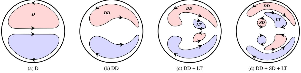
FIG. 9. Schematic of Dean (D), deformed Dean (DD), split Dean (SD) and Lyne-type (LT) vortex pairs viewed from upstream; clockwise and counter-clockwise rotation of the secondary flow are indicated by the arrows.
