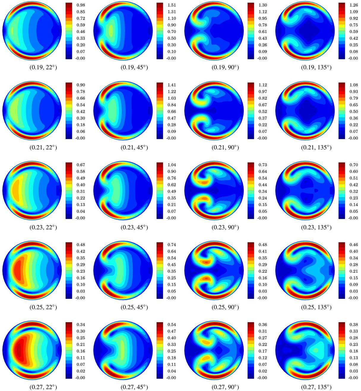
FIG. 7. Uniform entrance condition: nondimensional secondary velocity magnitude  $|\mathbf{u}_{\theta r}^*|$  at  $(t^*, \phi)$ . Different secondary flow patterns emerge along the curved cross-sections due to varying degrees of flow development, centrifugal forcing and flow reversal, although the lack of flow development at the entrance to the curvature inhibits secondary motion in the core and growth of interior flow vortices (see Sec. III B).
