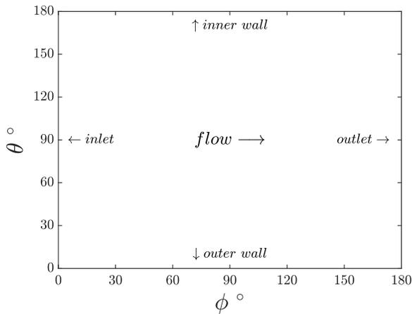
FIG. 15. Two-dimensional mapping of the upper wall of the curved section depicted in Fig. 1, indicating positive primary flow direction and location of the inlet, outlet and inner/outer wall. This mapping is used to visualize distribution of the instantaneous wall shear stress vector  $\tau_w^*$  over the entire surface.
