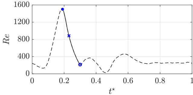
FIG. 2. Physiological (pulsatile) waveform in terms of Reynolds number  $Re$  as a function of nondimensional pulse period  $t^* = t/T$  (dash), displaying rapid deceleration (solid) during the interval  $0.19 < t^* < 0.30$ .  $Re|_{t^*=0.19} = 1501$  (blue dot),  $Re|_{t^*=0.23} = 883$  (blue cross),  $Re|_{t^*=0.30} = 215$  (blue circle).
