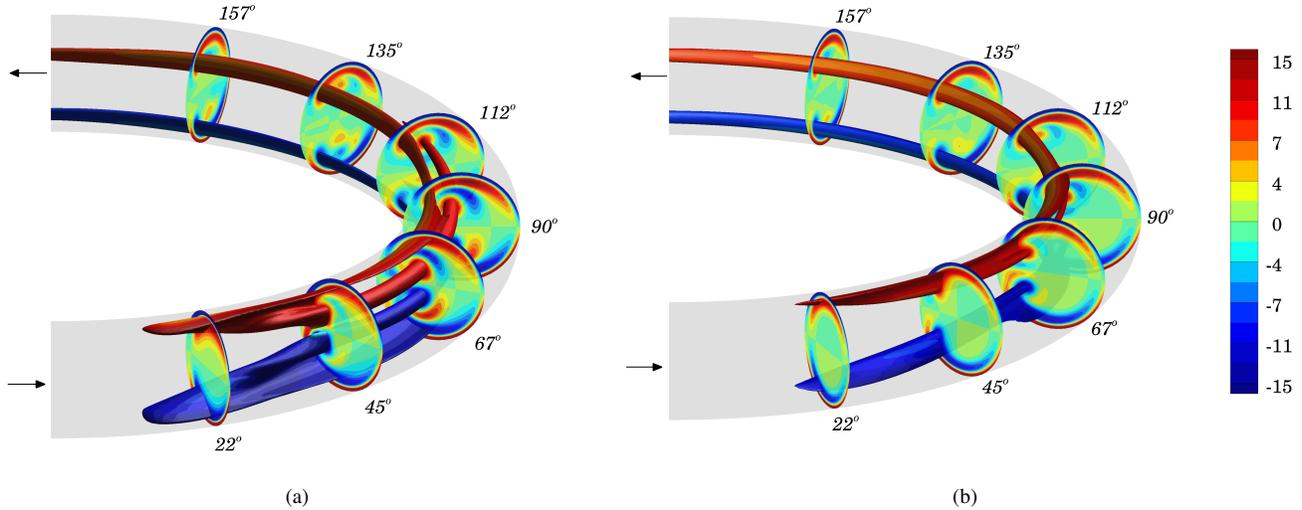
FIG. 14. Womersley and Uniform entrance conditions: isosurfaces of  $\lambda_2^* = -24$  colored by non-dimensional streamwise vorticity  $\omega_s^*$  at mid-deceleration phase  $t^* = 0.23$  under a) WEC and b) UEC. The helical streamlines displayed in Fig. 8, resulting from secondary flow, intensify streamwise vorticity and lead to a larger vortical structure and separation of the deformed-Dean “head” in a).
