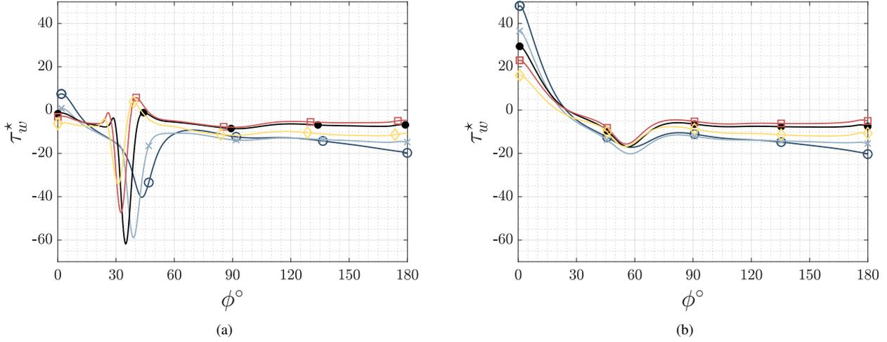
FIG. 17. Instantaneous wall shear stress  $\tau_w^*$  at the inner wall ( $\theta = 180^\circ$ ) as a function of toroidal position  $\phi$  under (a) WEC and (b) UEC for  $t^* = 0.23$  ( $\circ$ ),  $t^* = 0.24$  ( $\times$ ),  $t^* = 0.25$  ( $\bullet$ ),  $t^* = 0.26$  ( $\square$ ),  $t^* = 0.27$  ( $\diamond$ ). Under WEC, locally increased wall shear stresses occur in the range  $30^\circ < \phi < 45^\circ$ , with maximum  $|\tau_w^*|$  approximately four times larger than UEC.
