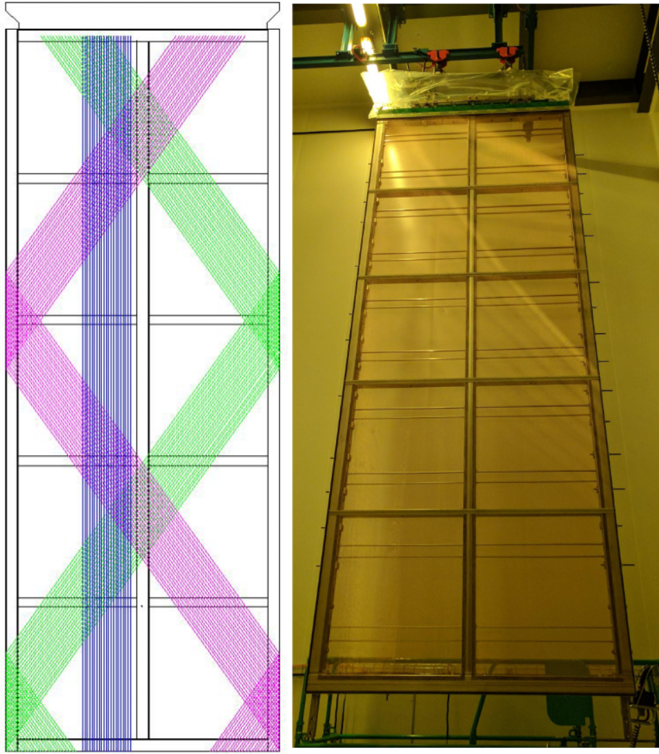
Figure 27: Left: Sketch of a ProtoDUNE-SP APA showing portions of the wire layers: the induction layers U (green) and V (magenta); and the collection layer X (blue). Only portions are shown to accentuate their angular relationships to the frame and to each other. The induction layers are connected electrically across both sides of the APA. The grid layer (G) wires (not shown), run vertically, parallel to the X layer wires; separate sets of G and X wires are strung on the two sides of the APA; they are not wrapped. The mesh is not shown. Right: Assembled APA hanging inside the clean room next to the ProtoDUNE-SP cryostat at CERN.
