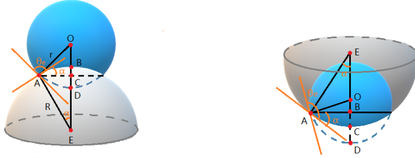
Figure 2: A droplet placed on the outside and inside surfaces of a larger sphere. Left: The negative mean curvature case( \kappa < 0 ); Right: The positive mean curvature case( \kappa > 0 ).
