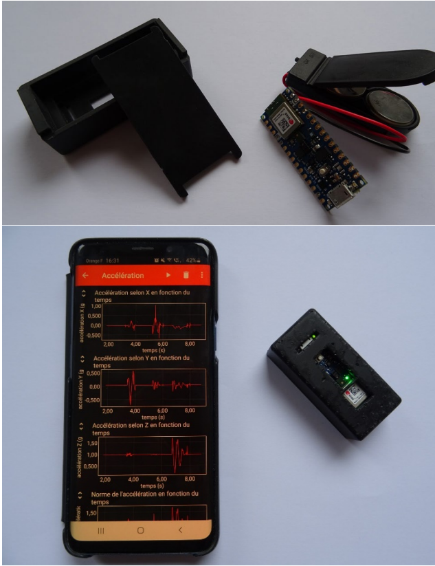
Figure 1: Top: the arduino nano bord connected to two button cells (right), next to a 3D printed case (left). Bottom: the arduino board and the button cells are in the case, transferring data to the smartphone via Bluetooth Low-Energy.
