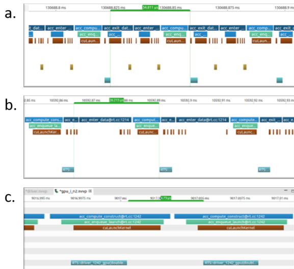
Figure 10: Nvprof profiler highlights the process of reducing kernel launch overhead in the RTS integrate() kernel. (a) Overhead between 2 launches, (b) Reduced overhead between kernels launches, and (c) Further reduced overhead
