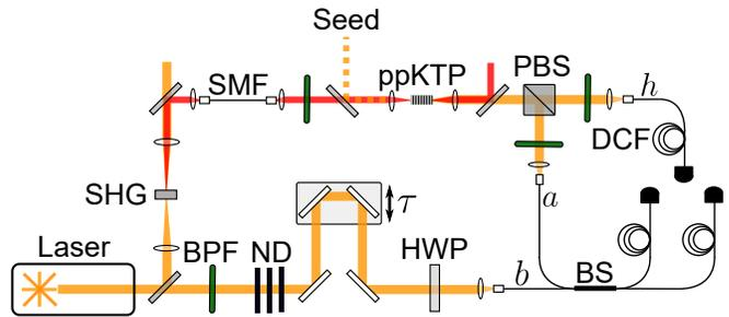
FIG. 2. Experimental setup. The SMF and seed are included only in certain measurements which are described in the main text. SHG: second-harmonic generation, SMF: single-mode fiber, BPF: bandpass filter, ND: neutral-density filter, ppKTP: periodically poled potassium titanyl phosphate, (P)BS: (polarizing) beam splitter, HWP: half-wave plate, DCF: dispersion-compensating fiber.
