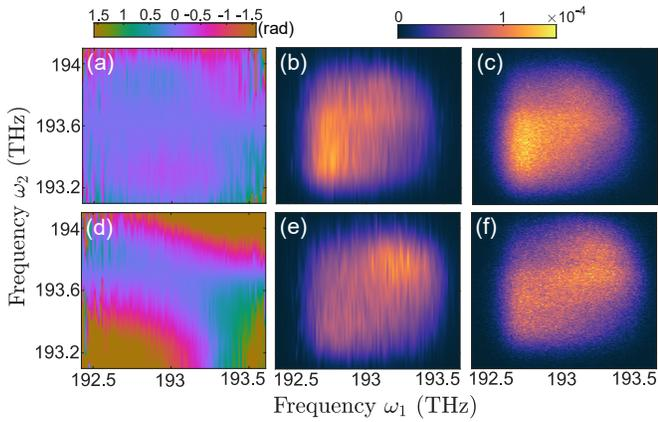
FIG. 3. Measured joint spectral amplitude. Top (bottom) row shows results with a chirpless (chirped) pump. (a) and (d) are the joint spectral phases  $\arg\{f(\omega_1, \omega_2)\}$  while (b) and (e) are the amplitudes  $|f(\omega_1, \omega_2)|$ . (c) and (f) are the amplitudes measured using a conventional phase-insensitive method.
