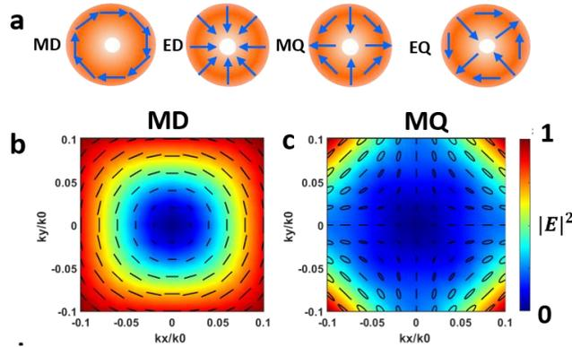
**Fig. S5.** (a) Schematic of far-field polarization vectors of different multipoles in the momentum space. MD, ED, MQ and EQ denote magnetic dipole, electric dipole, magnetic quadrupole and electric quadrupole, respectively. Calculated far-field vector and intensity distribution of the (b) MD and (c) MQ modes of the metasurface in the momentum space, which are illustrated in the manuscript.
