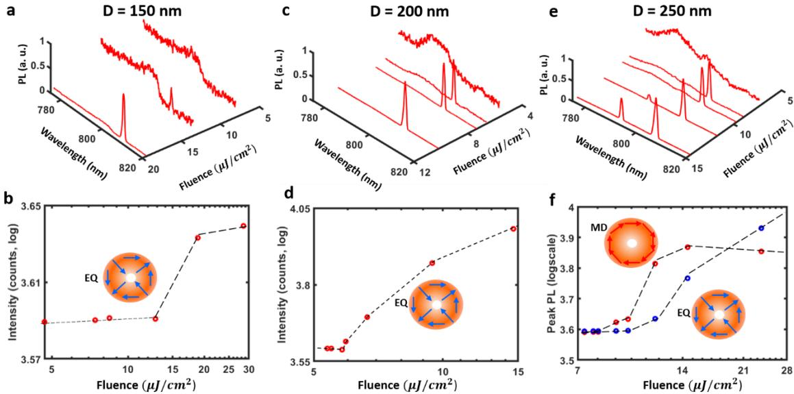
**Fig. S6.** Room-temperature emission spectra of the MAPbI<sub>3</sub> BIC metasurface and its Light-light curve with (a), (b)  $d = 150$  nm; (c), (d)  $d = 200$  nm and (e), (f)  $d = 250$  nm as function of pump fluence.
