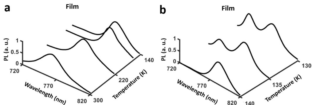
**Fig. S2.** Evolution of PL spectra from the MAPbI<sub>3</sub> film (a) from 298 K to 140 K and (b) from 140 K to 130 K.
