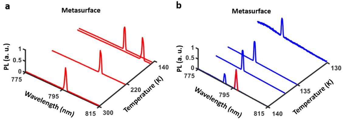
**Fig. S3.** Evolution of laser spectra from the MAPbI<sub>3</sub> metasurface (a) from 298 K to 140 K and (b) from 140 K to 130 K.
