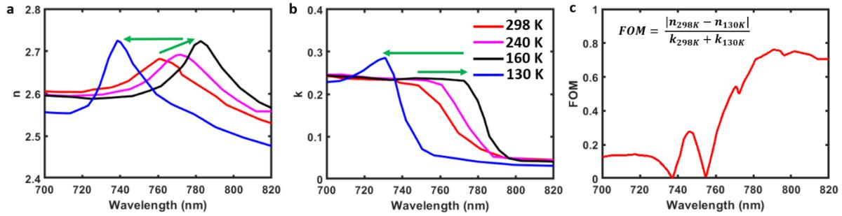
**Fig. S1.** (a) Real part and (b) imaginary part of refractive index of MAPbI<sub>3</sub> at different temperatures (22) (c) Phase-change figure of merit of MAPbI<sub>3</sub>.
