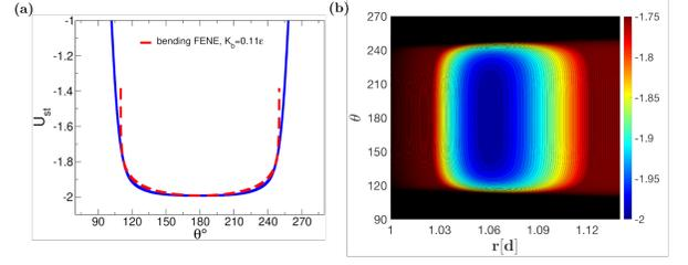
FIG. 6. (a) The potential energy profile for a 3-particle strand is shown in blue line and the fit of the bending FENE potential in red dashed line (b) The contour plot of the same energy  $U_{st}$  for different distances and angles with the color code representing the energy values.
