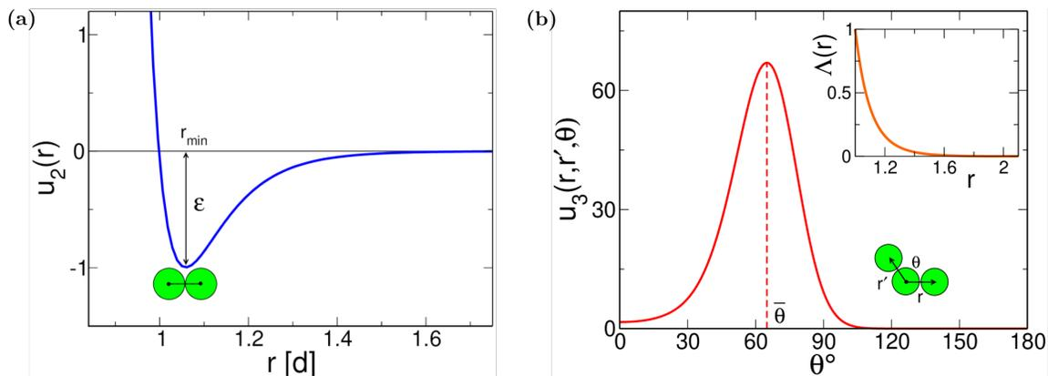
FIG. 2. (a) Two-body potential  $u_2$  as a function of distance between two particles,  $r$  in units of a particle diameter  $d$ , and (b) Main: Three-body interaction  $u_3$  for  $r = r' = r_{min}$  (both bonds at the minimum of the attractive well) and  $\bar{\theta} = 65^\circ$  as a function of angle between the neighboring bonds,  $\theta$ . Other parameters are  $B = 67.27$ , and  $w = 0.30$ . Inset: Radial modulation  $\Lambda(r)$  as a function of distance.
