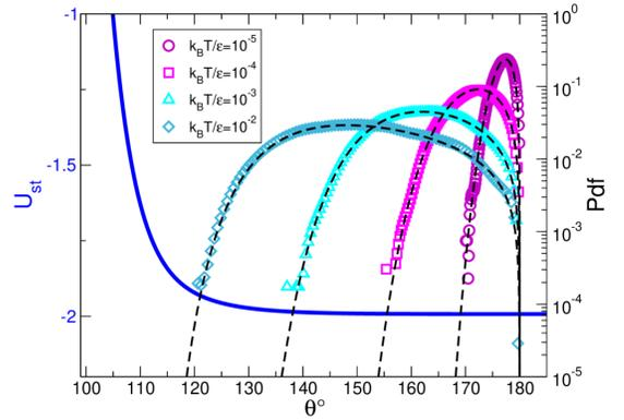
FIG. 7. The energy profile for  $U_{st}$  (left axis) in blue solid line. The bond angle distributions (right axis) for 3-particle strand for different thermal fluctuations. The dashed lines represent the prediction from Boltzmann probability distribution.
