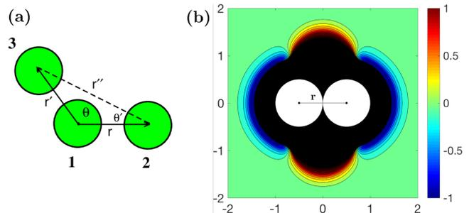
FIG. 3. (a) Illustration of the interactions for a particle **3** approaching two particles **1** and **2** previously bonded. (b) Contour plot of the potential energy experienced by an incoming particle when it approaches an existing bond at different distances and angles. The color is blue when the potential energy is  $-1$  and is red for  $+1$  or higher.
