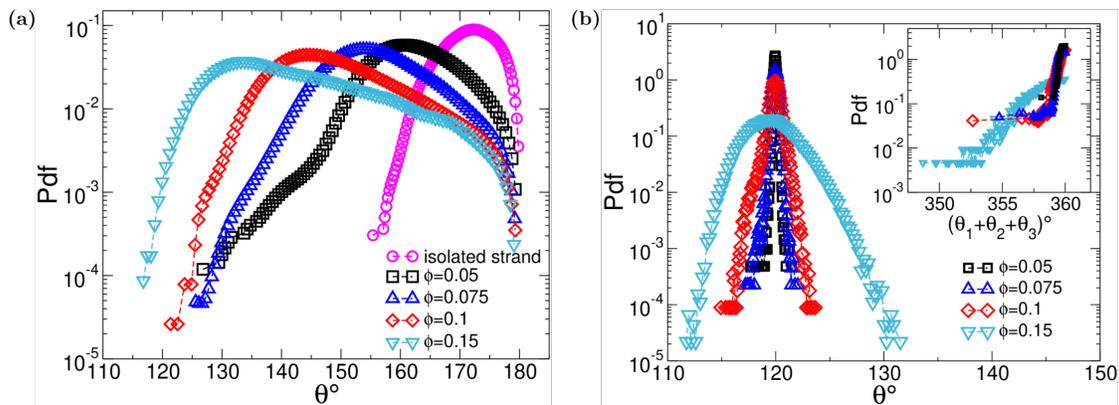
FIG. 10. (a) The distribution of bond angles for an isolated strand and for strands in networks at different volume fractions  $\phi$ . (b) Main: The distributions of bond angles that correspond to the branching points. Inset: The distribution of sum of three angles at a single branching point where the sum equal to  $360^\circ$  corresponds to a planar branching point.
