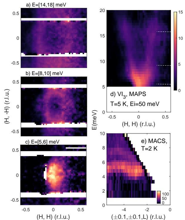
FIG. 2. (a – c)  $T=5$  K constant energy slices from MAPS. Energy integration ranges for each of the cuts in panels (a – c) are given in square brackets. (d) Momentum-energy slice illustrating dispersive modes from  $Q=0$ . The locations of the constant energy slices are given by the dashed white lines. (e) The excitations along the  $c$ -axis from MACS.  $L$  introduction is discussed in the SI. [34]
