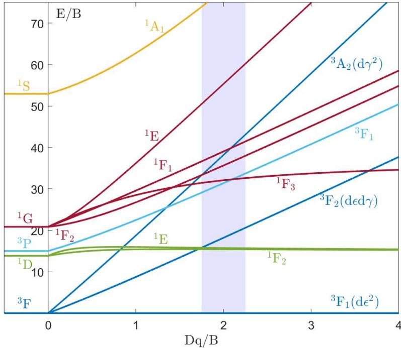
FIG. 8. Tanabe-Sugano diagram for a  $d^2$  ion showing the splitting due to an octahedral field, with a  $C/B = 4.42$  as appropriate for  $V^{3+}$ . Corresponding strong crystal field bases are labeled in parentheses. The blue shaded region indicates the ratio  $Dq/B \approx 2$  that one expects for  $V^{3+}$  [7].
