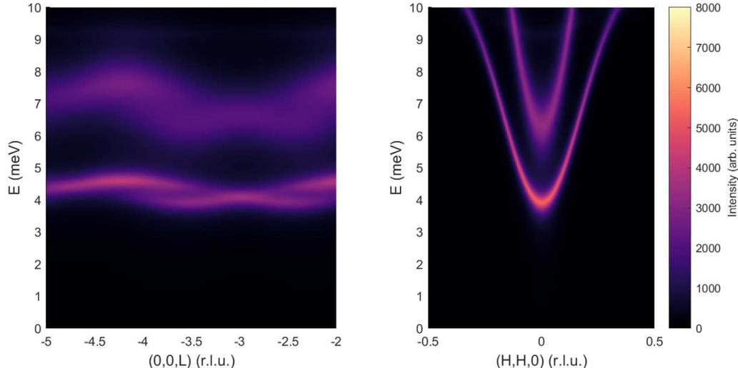
FIG. 7. (a) Calculated dispersion along L with the fitted values from the main text and a small coupling along  $c$  ( $J_c = -0.5$  meV). (b) The calculated in-plane dispersion with coupling along  $c$ , showing a small change in the gap to the lower mode ( $\sim 0.4$  meV), but no significant change in the spectrum.
