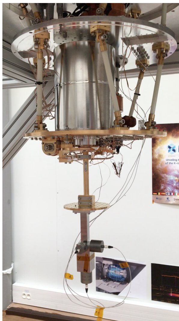
Fig 3 The interior of the Elsa cryostat, showing the three piezo-accelerometers mounted onto the 50 mK cold stage.
