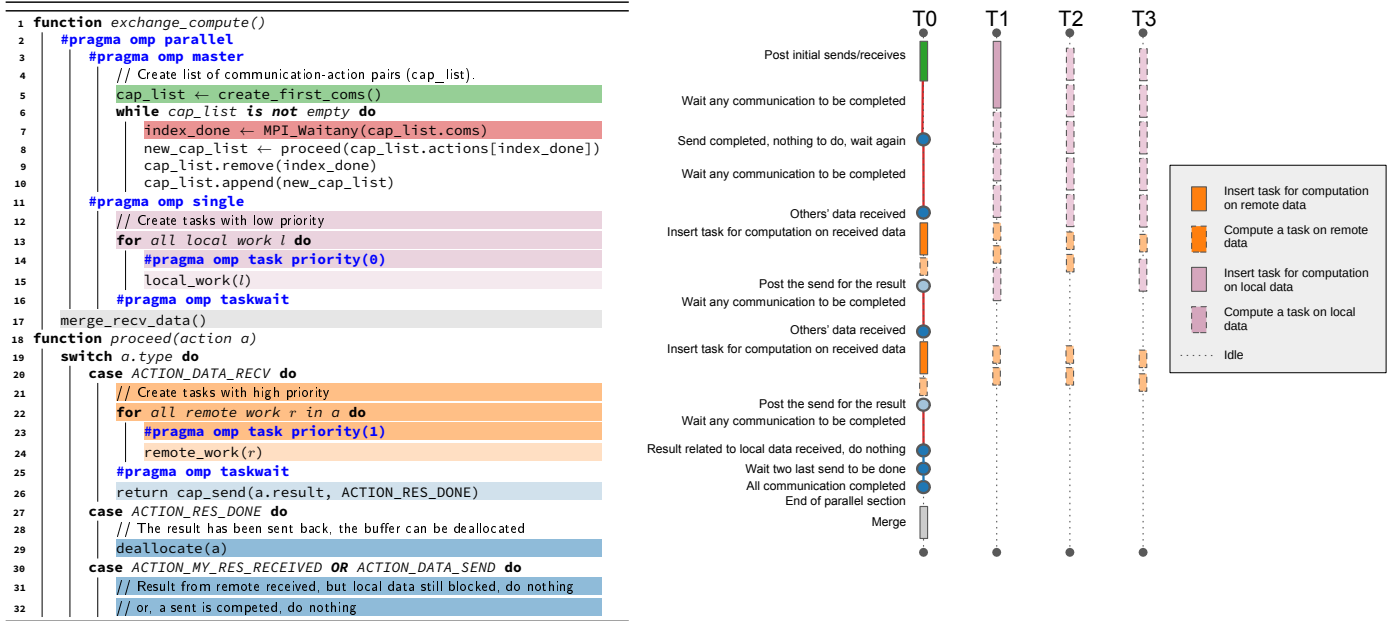
Figure 2: Overview of parallel interpolation algorithm (left) and reference execution timeline for one process with four threads (right). Colored lines of code correspond to individual timeline elements. The threads compute local operations by default but switch to remote operations when the master thread creates the corresponding new higher-priority tasks. With the use of priorities, the execution pattern allows for quicker communication of results to different processes. See text for details.
