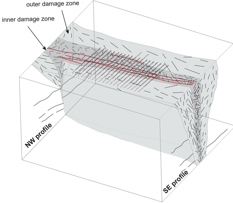
Figure 5. Schematic illustration of the fault zone at SGB site. Black dots refer to the geophones and red lines represent the Clark fault traces.
