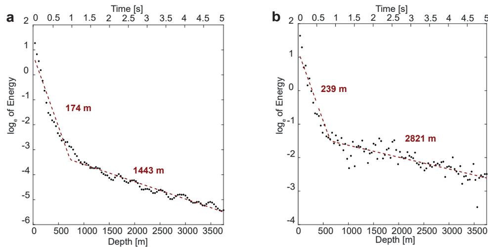
Figure S3. Mean intensity decay as a function of depth with the corresponding linear regression in logarithmic scale and the characteristic length of decay values. (a) Intensity decay of raw images. (b) Intensity decay of images corrected from the aberrating component.
