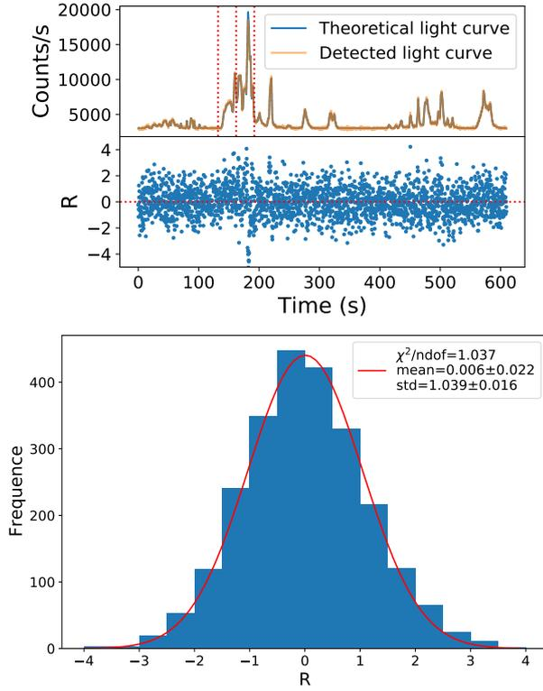
**Fig. 11** Upper: The upper panel is the “super-long” curve synthesized with several actual GRBs observed by *Fermi*/GBM (blue line), then reproduced by the GRB simulator and detected by GRDs (orange line). GRD#5, #6, #13, #14, #15, #16, #22, #23 and #24 were selected. The bottom panel is the residual of theoretical curve and detected light curve. Bottom: The distribution of the residual. The red line is the result of Gaussian fitting.
