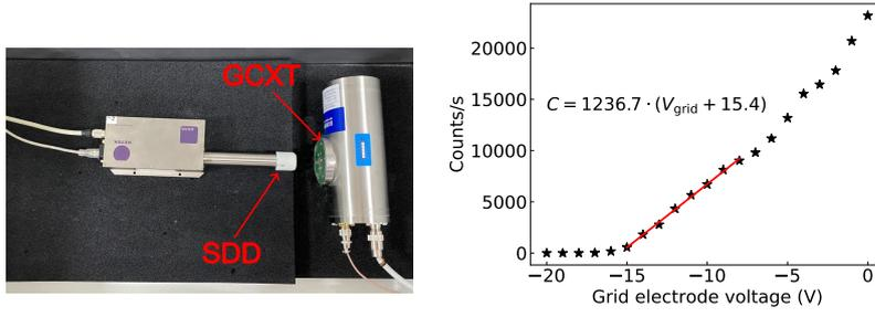
**Fig. 5** Left: Experimental layout to investigate the modulation properties of GCXT. Right: Output count rates of GCXT versus grid electrode voltage.
