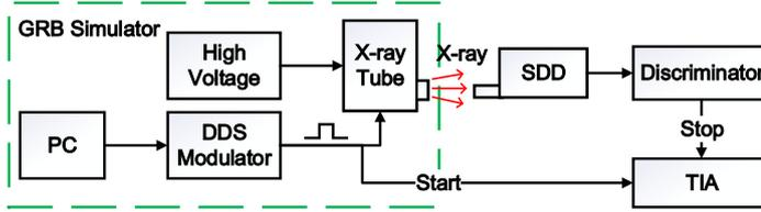
**Fig. 7** Simplified experimental schematic to investigate the time response of GCXT.
