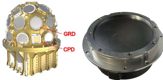
**Fig. 1** Left: Each GECAM satellite is equipped with 25 GRDs and 8 CPDs. Right: The photo of a GRD of GECAM.
