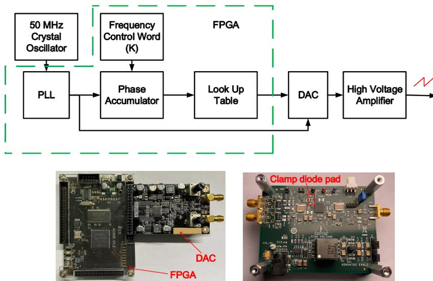
**Fig. 3** Upper: Simplified schematic of DDS modulator. Lower-left: Circuit board of FPGA and DAC. Lower-right: ADI ADHV4702-1 high-voltage precision operational amplifier board whose clamp diode is removed to maximize slew rate.
