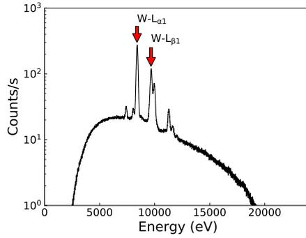
**Fig. 6** The raw energy distribution of GCXT detected by KETEK SDD when the high voltage source is set to 20 kV. The characteristic emission line of tungsten can be clearly seen, including the 8.40 keV W-L $_{\alpha 1}$  line and the 9.67 keV W-L $_{\beta 1}$  line.
