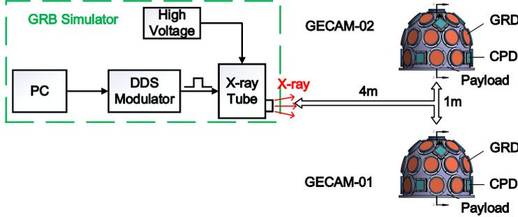
**Fig. 9** The layout of the ground GRB experimental to GECAM. GCXT is placed at the perpendicular bisector of GECAM-01 and GECAM-02 with about 4 m away from two satellites to allow X-rays to irradiating two satellites at the same time. The distance between the center of the two satellites is 1 m.
