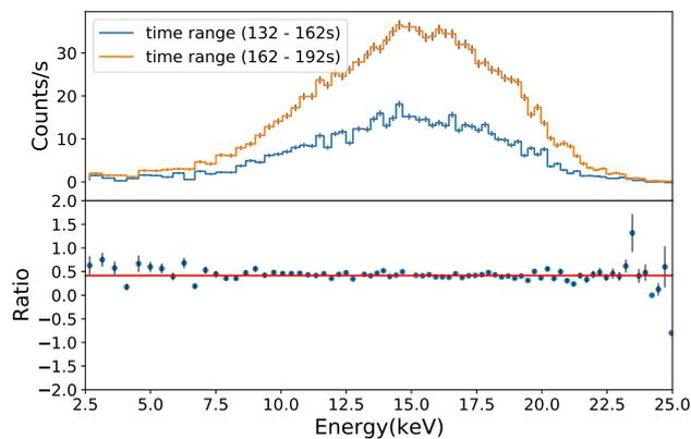
**Fig. 12** The shape of the energy spectrum detected by GRD in a different time range of super-long GRB (in Fig. 11) is consistent which illustrates the good energy spectrum stability of the device over time.
