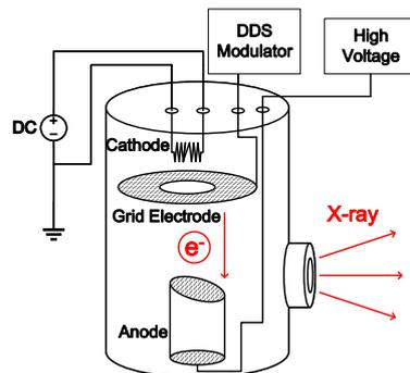
**Fig. 4** Simplified schematic of the GCXT, mainly composed of cathode, grid electrode and anode.
