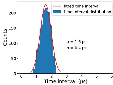
**Fig. 8** Time delay and time jitter of the GRB simulator. The blue line represents the detected time interval. The red line is the result of Gaussian fitting.
