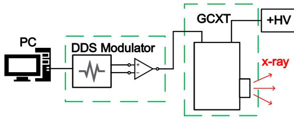
**Fig. 2** Schematic of the GRB simulator mainly consist of DDS modulator and GCXT.
