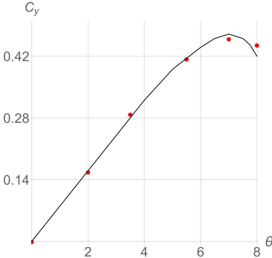
Fig. 5. Comparison of calculations of the dependence of lift force on the angle of attack.
