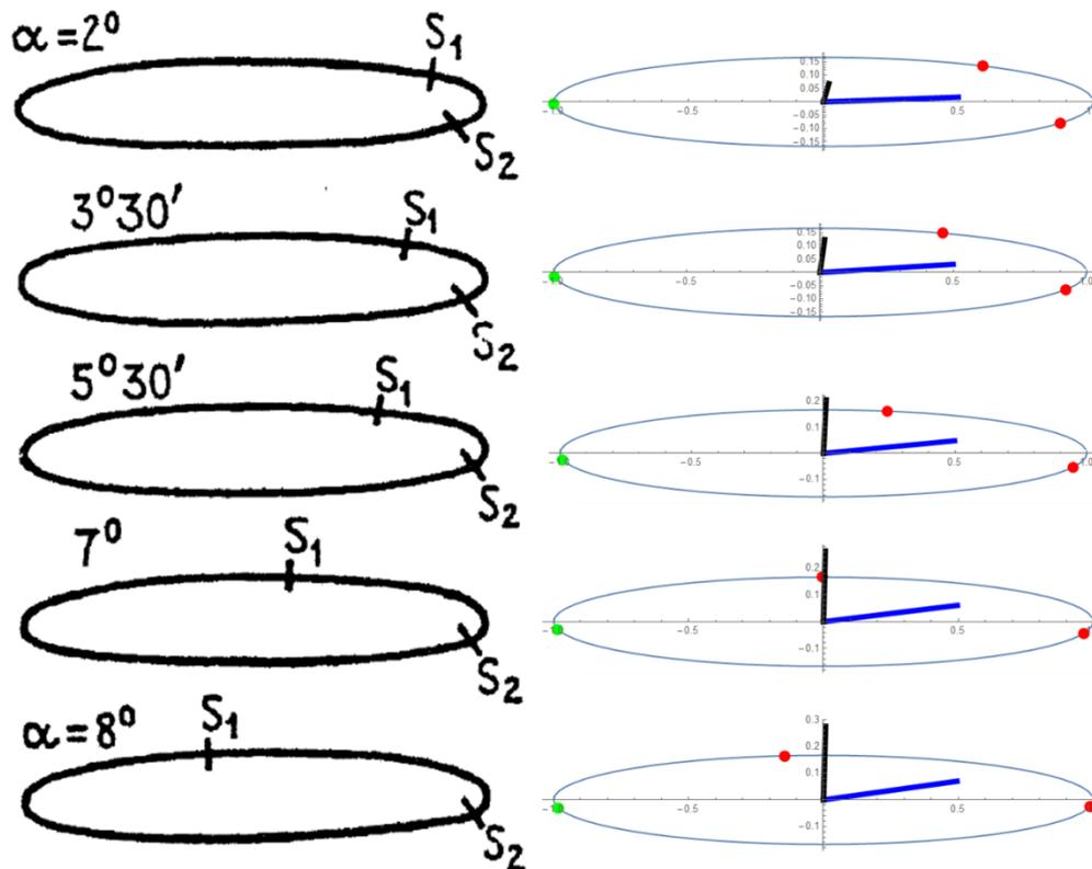
Fig 4. Separation points in case of the ellipse axis ratio 6:1 under different angles of attack.
