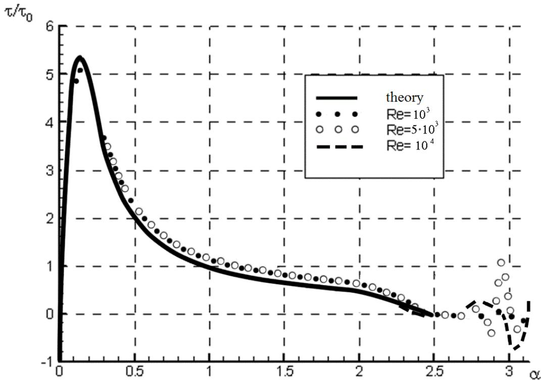
Fig. 2. Comparison with direct numerical solution of the Navier-Stokes equations for different Reynolds numbers
