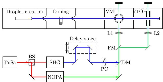
FIG. 2. Schematic drawing of the experimental setup. Abbreviations: Ti:Sa = titanium:sapphire laser system, BS = nonpolarizing beamsplitter, SHG =  $\beta$ -barium borate crystal for second harmonic generation, NOPA = nonlinear optical parametric amplifier, PC = prism compressor, DM = dichroic mirror, FM = flip mirror, L1 and L2 = lenses with a focal length of  $75\ \text{cm}$  each, VMI = velocity map imaging spectrometer, iTOF = ion time-of-flight mass spectrometer.
