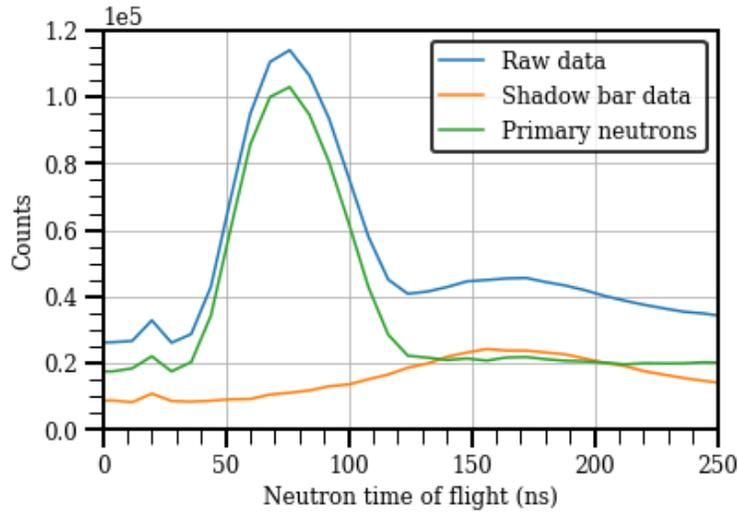
Figure 7: Distribution of neutron flight times for the raw data, the shadow-bar data, and the shadow-bar data subtracted from the raw data, i.e., only the primary neutrons.
