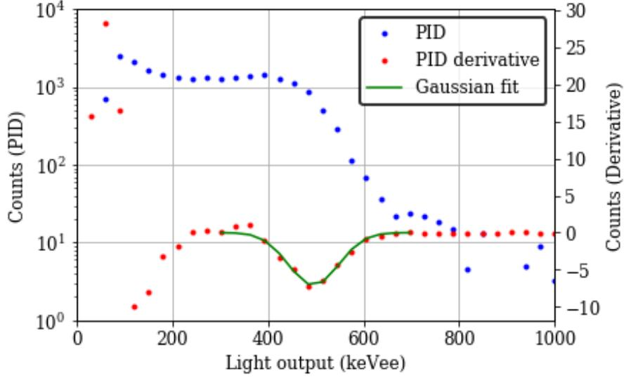
Figure 9: The PID as a function of the light output (LO), its derivative, and the Gaussian fit to find the minimum of the derivative, for the energy bin centered at 3.4 MeV. The equation of this Gaussian fit is  $y = -7.11e^{-\frac{(LO-495.84)^2}{2(52.45)^2}}$ .
