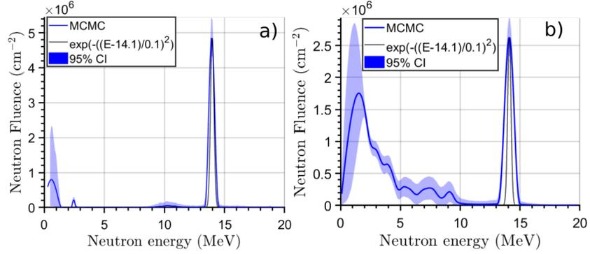
Figure 12: Results from unfolding the spectrum of a DT fusion source for (a) stilbene-d<sub>12</sub> and (b) <sup>1</sup>H-stilbene. The reference spectrum is normalized to the maximum of the distributions and shown for comparison purposes.
