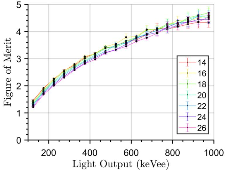
Figure 2: Stilbene-d<sub>12</sub> figures of merit as a function of light output for different values of  $t_{start}$  in ns.
