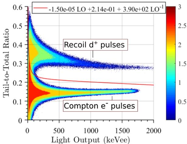
Figure 6: PSD of  $^{252}\text{Cf}$  source measured with the stilbene- $\text{d}_{12}$  detector. The PSD discrimination equation as a function of pulse light output (LO) was used to select neutron pulses. The colorbar indicates the number of pulses in logarithmic scale.
