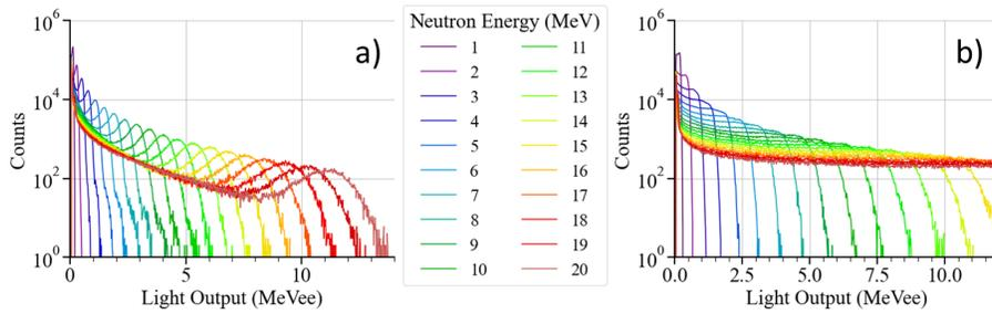
Figure 11: Simulated response matrix of (a) stilbene-d<sub>12</sub> and (b) <sup>1</sup>H-stilbene on a logarithmic scale, using MCNPX-PoliMi.
