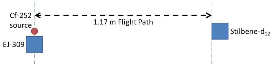
Figure 3: Schematic of the experimental setup used to determine the neutron light output response of the stilbene-d<sub>12</sub> detector through TOF.
