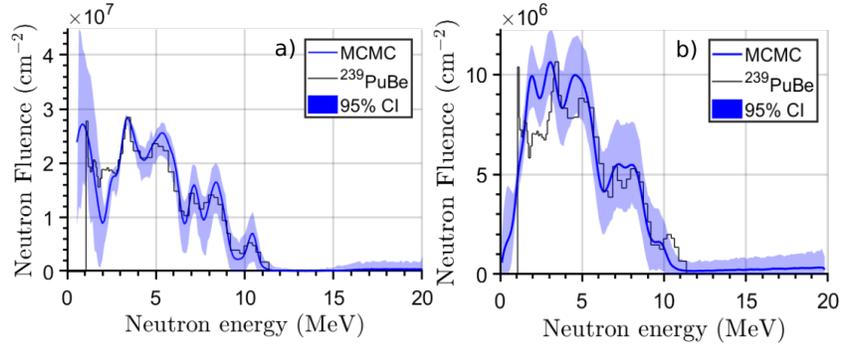
Figure 13: Results from unfolding the spectrum of a <sup>239</sup>PuBe fusion source for stilbene-d<sub>12</sub> (a) and <sup>1</sup>H-stilbene (b). The reference spectrum is normalized to the maximum of the distributions and shown for comparison purposes.
