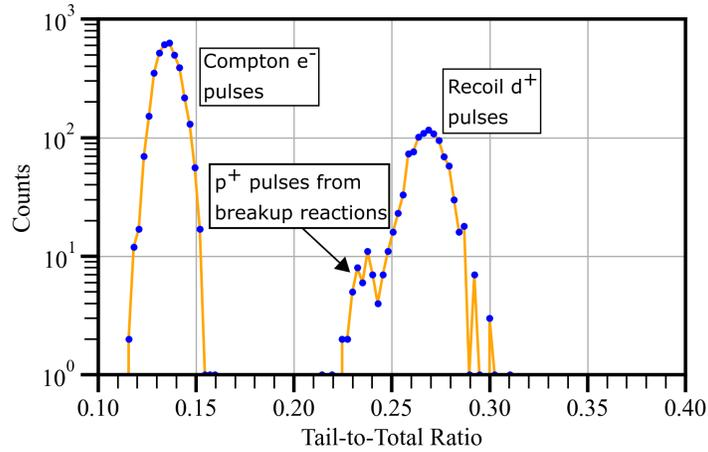
Figure 5: Slice of the PSD plot from the <sup>239</sup>PuBe source shown in Fig. 4, from 2025 keVee to 2292 keVee. A small peak from protons is visible next to the deuteron recoil peak.
