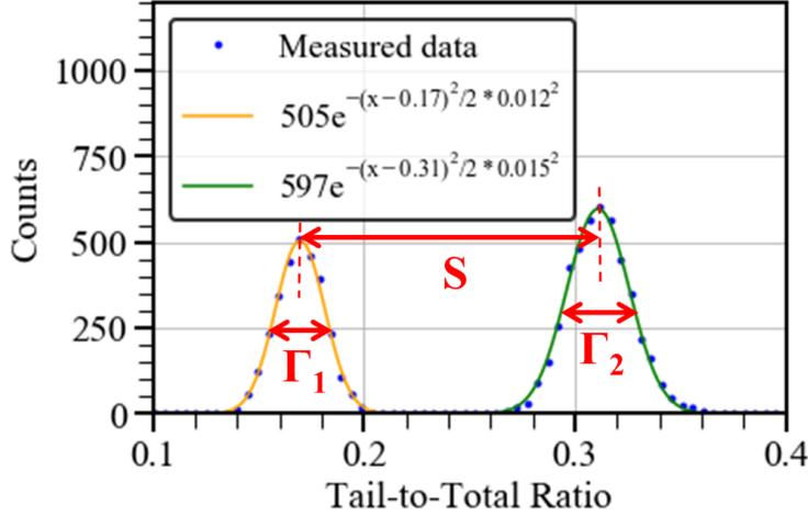
Figure 1: Distribution of  $^{239}\text{PuBe}$  counts in terms of tail-to-total ratio, in the 710-822 keVee light output interval. The gamma-ray peak is centered at 0.17 and the neutron peak is centered at 0.31.
