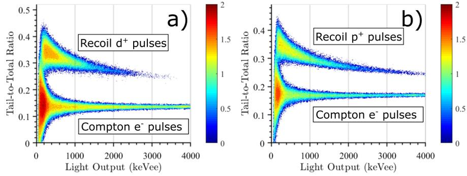
Figure 4: PSD of (a) stilbene-d<sub>12</sub> and (b) <sup>1</sup>H-stilbene for a <sup>239</sup>PuBe source. The colorbar indicates the number of pulses in a logarithmic scale.
