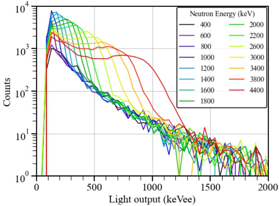
Figure 8: Response matrix of the stilbene-d<sub>12</sub> detector. Each curve is the light-output response to neutrons in a quasi-monoenergetic interval.
