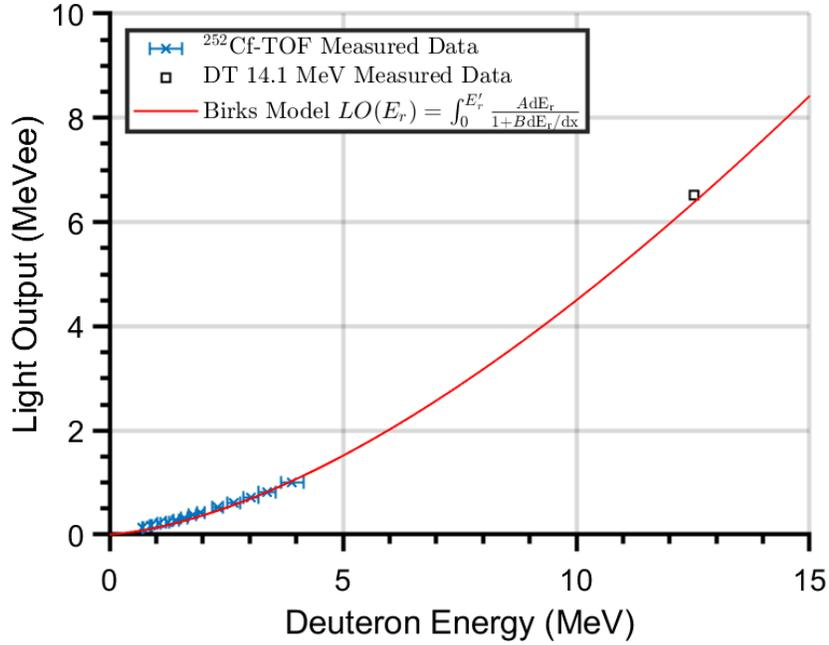
Figure 10: Light output curve of stilbene-d<sub>12</sub> with fitted Birks' model.
