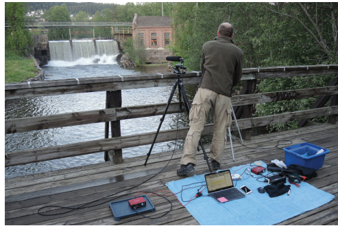
FIG. 5. Experimental setup with two microphones directed towards the center of the waterfall.
