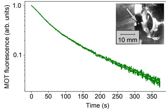
FIG. 2. Fluorescence decay of the MOT. An exponential decay fit at long times (white dashed line) gives a  $1/e$  decay time of about 140 s. The inset shows the MOT cloud (arrow) facing one of the aspheric lenses.
