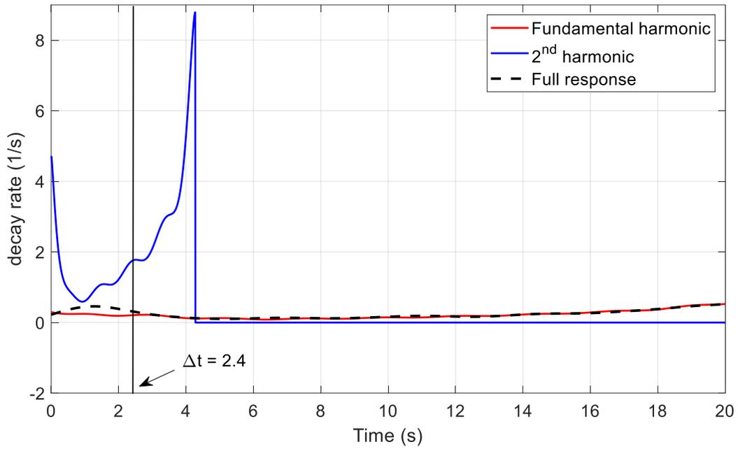
Extended Data Fig. 2. Decay rates of harmonics – Case 2. The black, the red and the blue curves represent the instantaneous decay rate of the full signal, fundamental and second harmonic, respectively, of the experimental measurements depicted in Ext. Data Fig. 1.
