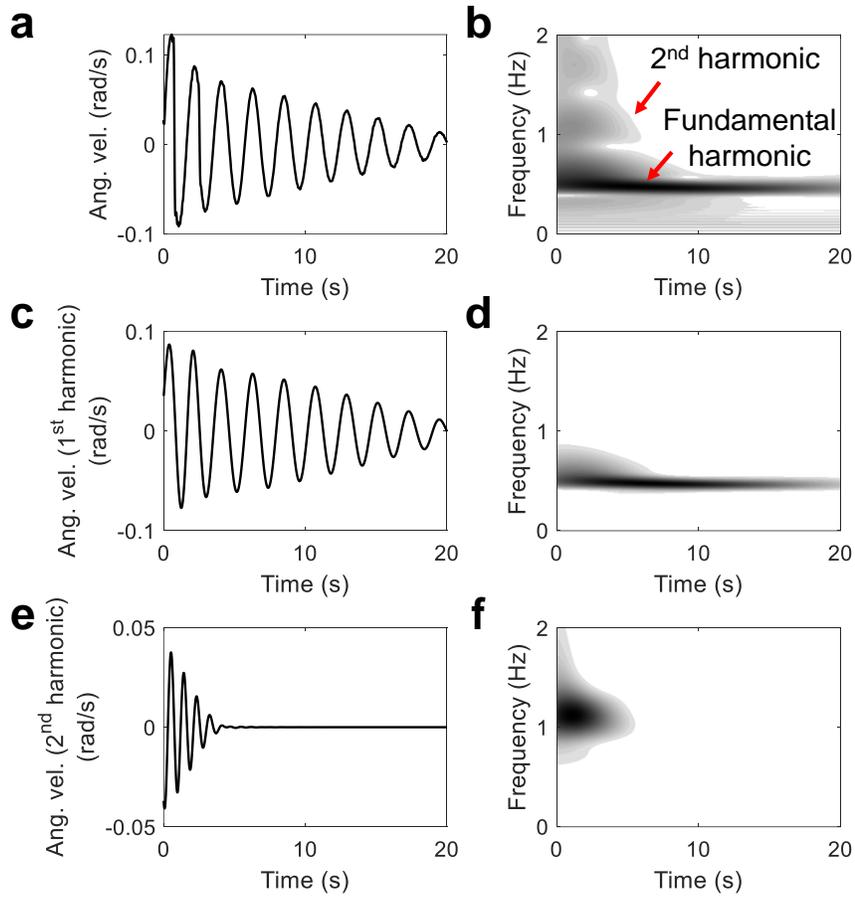
Extended Data Fig. 1. Harmonic separation – Case 2. Response of the experimental system excited by normalized input energy of  $\sim 10^{-2} \text{ J kg}^{-1} \text{ m}^{-2}$  in (a) the time domain and (b) with its corresponding wavelet spectrum. (c) and (d) show the time series and the wavelet spectrum of the fundamental harmonic, respectively. (e) and (f) show the time series and the wavelet spectrum of the second harmonic, respectively.
