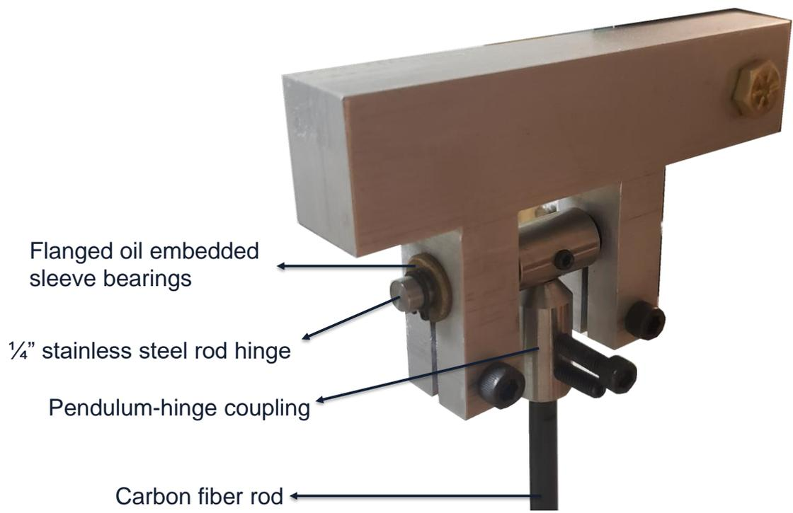
Extended Data Fig. 5. Configuration of the pendulum mount and pivot. Fully assembled mount of the pendulum, along with the hinge from which it hangs.
