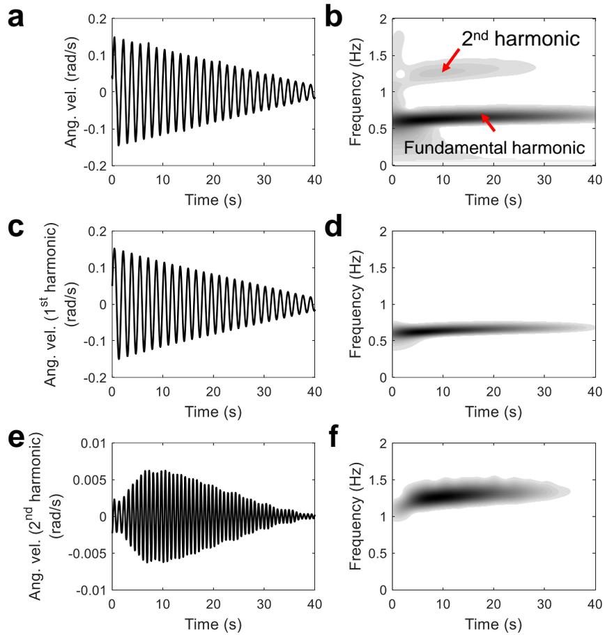
Extended Data Fig. 3. Harmonic separation – Case 3. Response of the experimental system excited by normalized input energy of  $\sim 10^{-2} \text{ J kg}^{-1} \text{ m}^{-2}$  in (a) the time domain and (b) with its corresponding wavelet spectrum. (c) and (d) shown the time series and the wavelet spectrum of the fundamental harmonic, respectively. (e) and (f) show the time series and the wavelet spectrum of the second harmonic, respectively.
