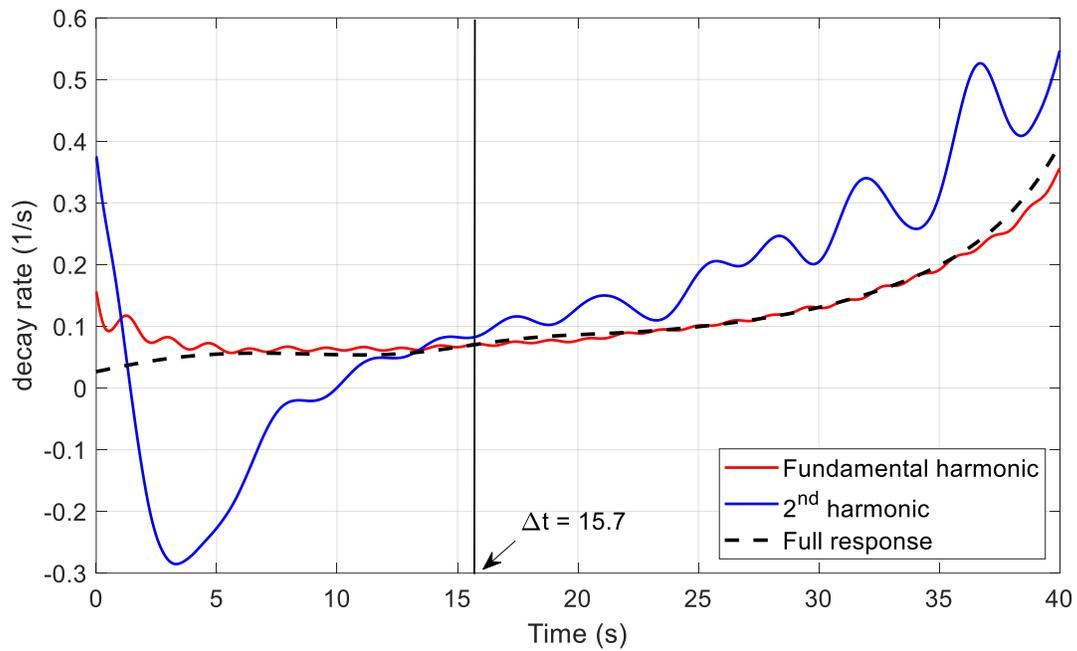
Extended Data Fig. 4. Decay rates of harmonics – Case 3. The black, the red and the blue curves represent the instantaneous decay rate of the full signal, fundamental and second harmonic, respectively, of the experimental measurements depicted in Ext. Data Fig. 3.
