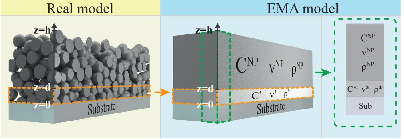
FIG. 8. Left: 3D nanoparticles thin film of thickness  $d$  adhered on a semi-infinite substrate. Centre: EMA model: *effective* NP layer ( $d < z < h$ ); *effective* interface layer ( $0 < z < d$ ); semi-infinite substrate ( $z < 0$ ). The NP layer is the same one addressed in the pillar model. The interface layer has effective mechanical properties  $C^*$ ,  $v^*$  and  $\rho^*$  (see text). The image is for illustrative purposes. Right: 1D sketch of the EMA model.
