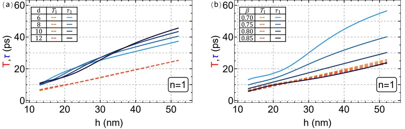
FIG. 10.  $T_1(h; d, \beta)$  and  $\tau_1(h; d, \beta)$  vs  $h$  for  $n = 1$  for the Ag nanogranular film: (a) fixed  $\beta = 0.73$  while varying  $d$  (expressed in nm); (b) fixed  $d = 12$  nm while varying  $\beta$ .
