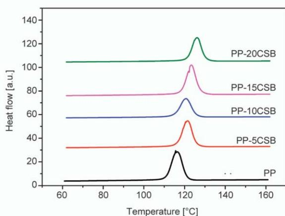
**Figure 12.** Crystallisation curve of PP/CSB composites.
