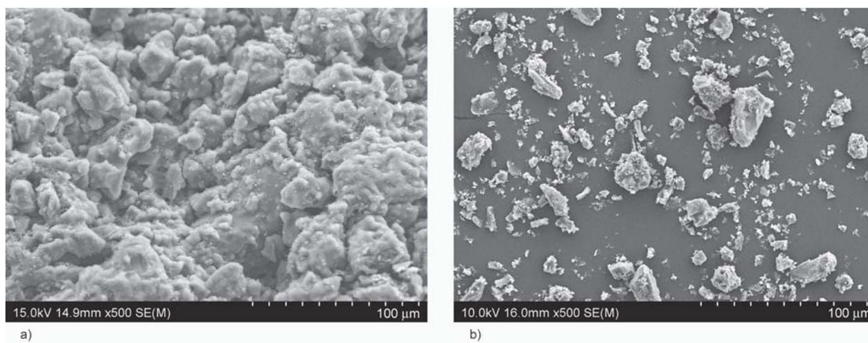
**Figure 1.** SEM images of CSB (a) before milling, and (b) after milling.
