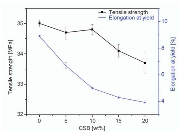
**Figure 6.** Tensile strength and elongation at yield of PP/CSB composites with varying biocarbon percentage.
