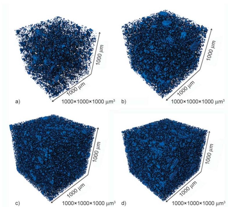
**Figure 9.** Micro-CT CSB particles distribution of (a) PP-5CSB (b) PP-10CSB (c) PP-15CSB (d) PP-20CSB.
