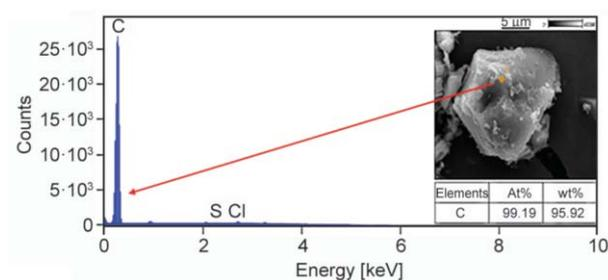
**Figure 2.** Energy dispersive spectroscopy (EDS) analysis of CSB.
