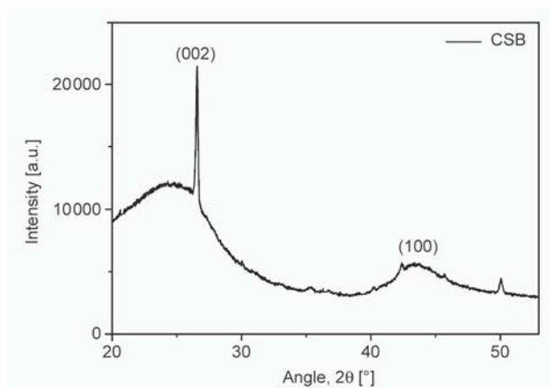
**Figure 4.** X-ray Diffraction analysis of CSB.
