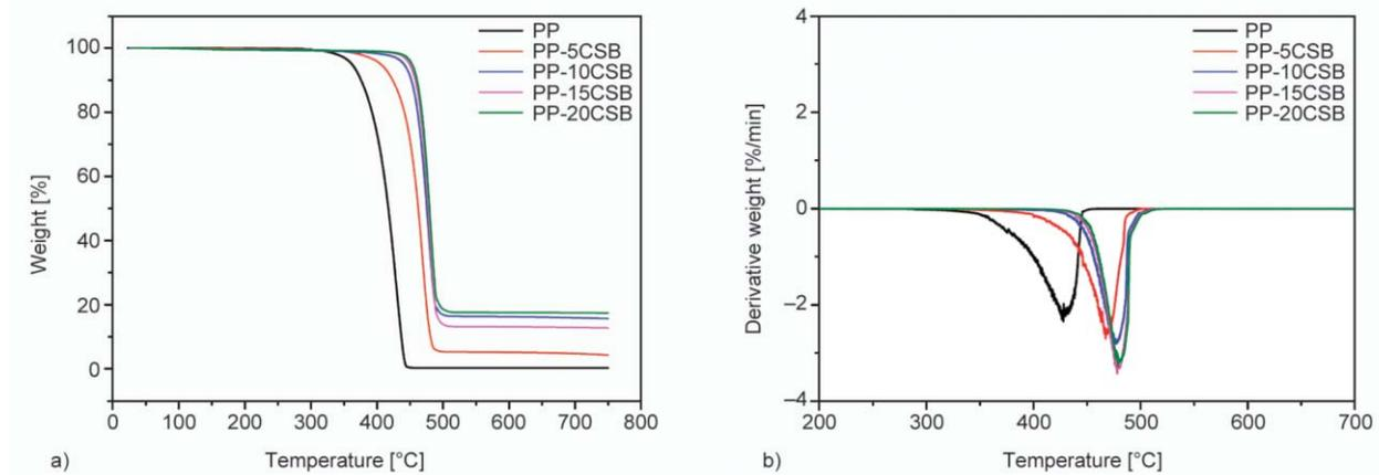
**Figure 13.** (a) TGA and (b) DTG curve of PP/CSB composites.
