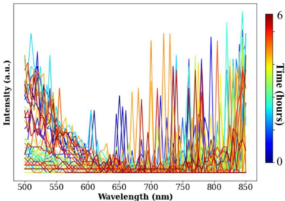
**Figure S3:** PL spectrum of  $\text{MA}_{0.20}\text{Cs}_{0.80}\text{Pb}(\text{I}_{0.20}\text{Br}_{0.80})_3$ . Absence of a defined peak, indicating the rapid degradation of  $\text{CsPbBr}_3$ -rich compositions when toluene is used as the antisolvent.
