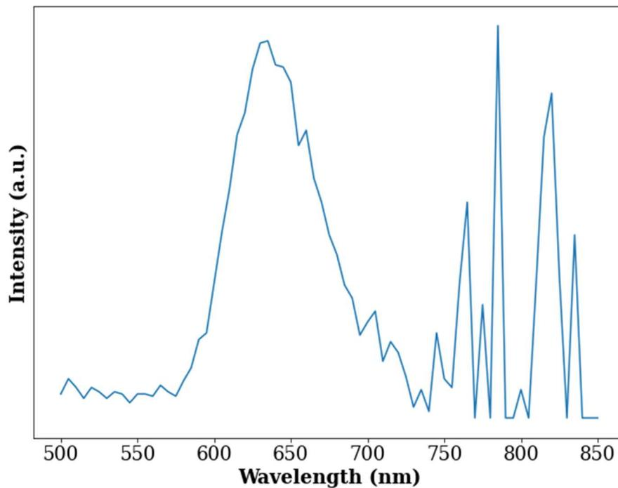
**Figure S2: PL spectrum of FAPbI<sub>3</sub>.** Observed a broad peak around 650 nm, indicating the formation of the photoinactive, yellow phase ( $\delta$ -FAPbI<sub>3</sub>).
