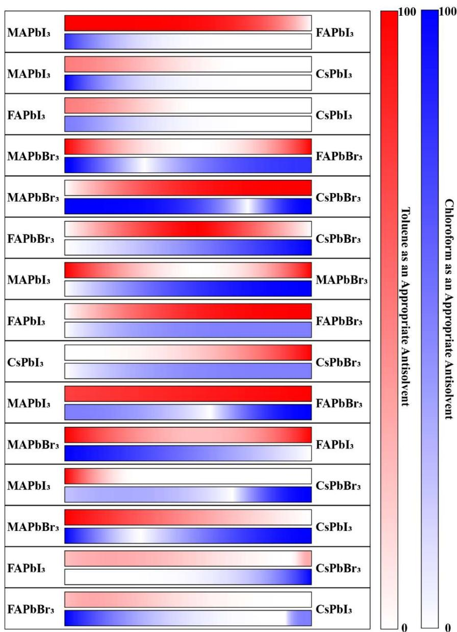
**Figure 6. Assessment for which antisolvent is more applicable for each system.** White or light red/blue indicate the antisolvent is not ideal for that section of the phase diagram as the microcrystals either form different phases or exhibit poor stability. As the color darkens, this indicates the antisolvent is an appropriate choice for the portion of the phase diagram as the correct phase forms and remains stable for longer periods of time.
