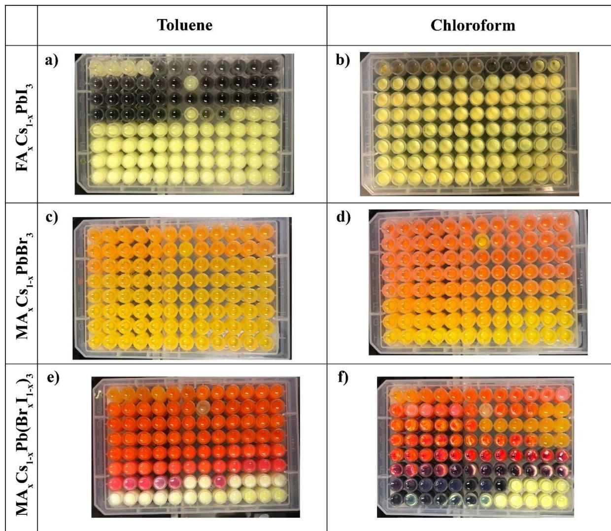
**Figure S1.** Photographs of the microplates when a), c), and e) toluene and b), d), and f) chloroform is used as the antisolvent for  $\text{FA}_x\text{Cs}_{1-x}\text{PbI}_3$ ,  $\text{MA}_x\text{Cs}_{1-x}\text{PbBr}_3$ , and  $\text{MA}_x\text{Cs}_{1-x}\text{Pb}(\text{BrI}_{1-x})_3$  systems, respectively.
