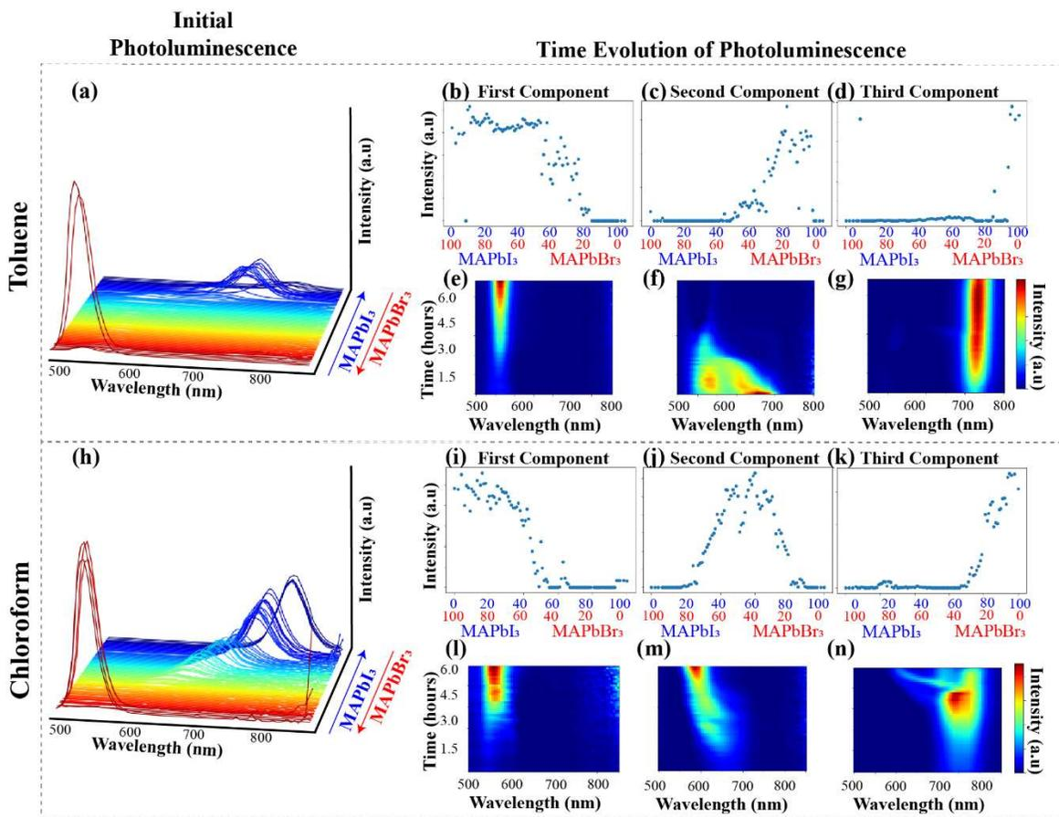
**Figure 3. Methylammonium lead double halide system, MAPb(I<sub>x</sub>Br<sub>1-x</sub>)<sub>3</sub>.** a) initial PL behavior when toluene is used as the antisolvent. b), c), and d) are the loading maps for MAPbBr<sub>3</sub>-rich compositions, solid solutions of MAPbBr<sub>3</sub> and MAPbI<sub>3</sub>, and MAPbI<sub>3</sub>-rich compositions,
