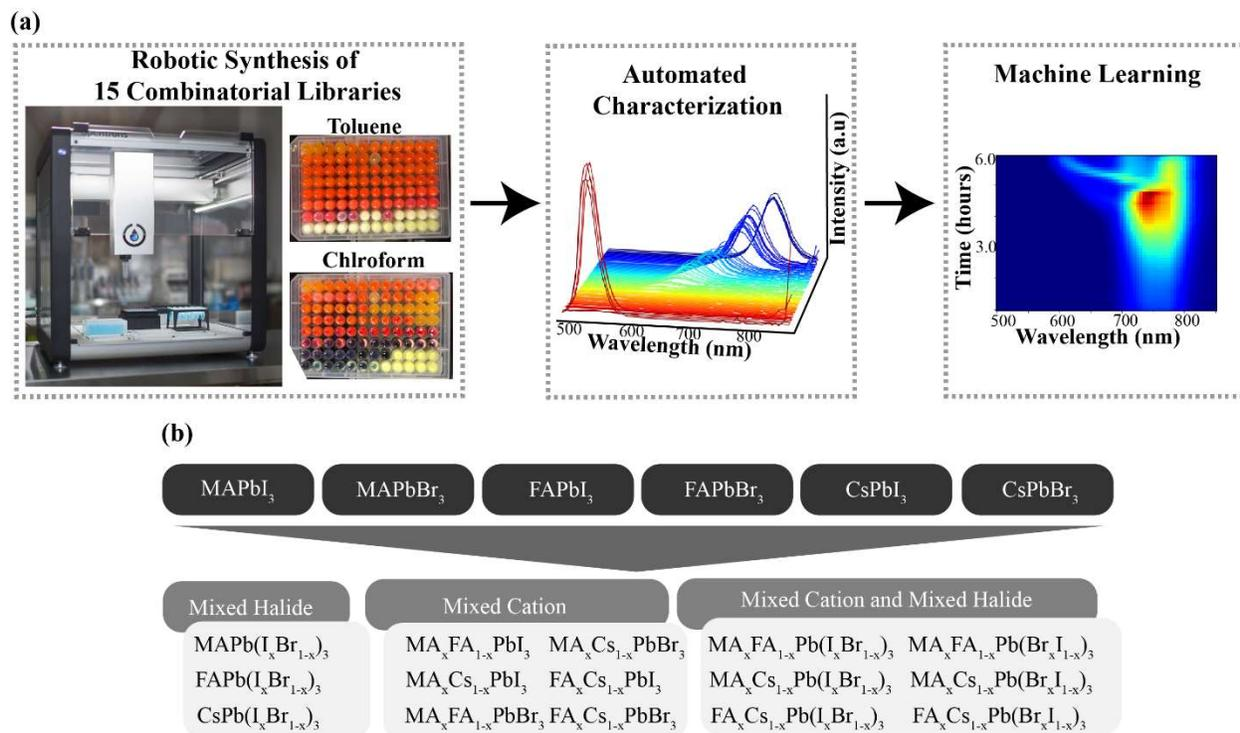
**Figure 1.** a) Schematic of the experimental workflow utilized for the exploration of 15 combinatorial libraries. We utilize robotic synthesis to fabricate a library twice with two different solvents: toluene and chloroform, photoluminescence (PL) spectroscopy is automatically performed next. Finally, we utilize machine learning to effectively map characteristic PL behaviors
