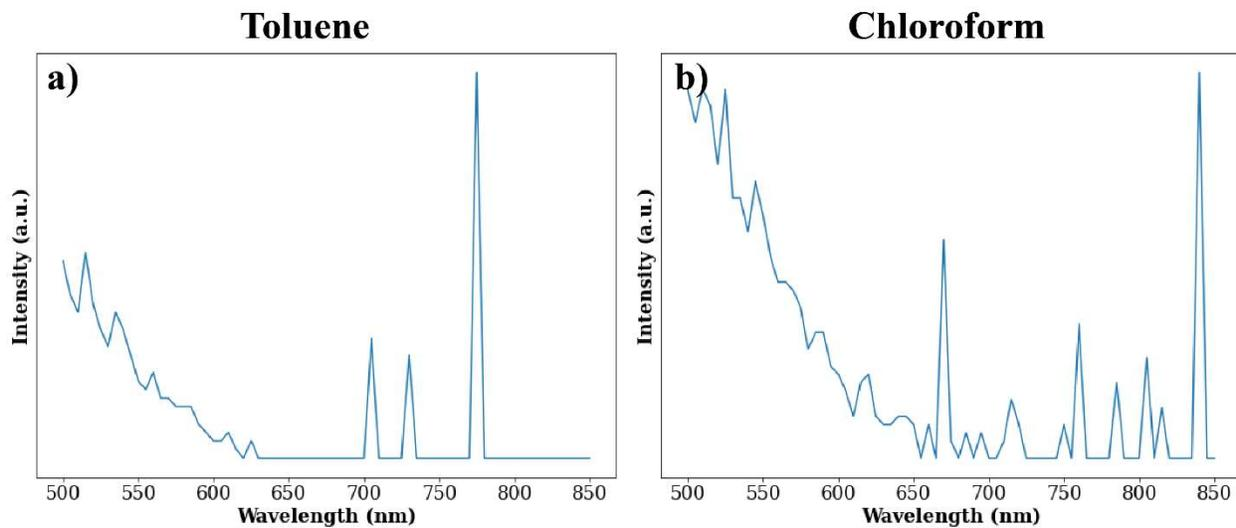
**Figure S4:** PL spectra of  $\text{CsPbI}_3$  when a) toluene and b) chloroform is used as the antisolvent. Notably, we observe a broad peak at lower wavelengths, indicating the formation of the wide-band gap, polymorph  $\delta\text{-CsPbI}_3$ .
