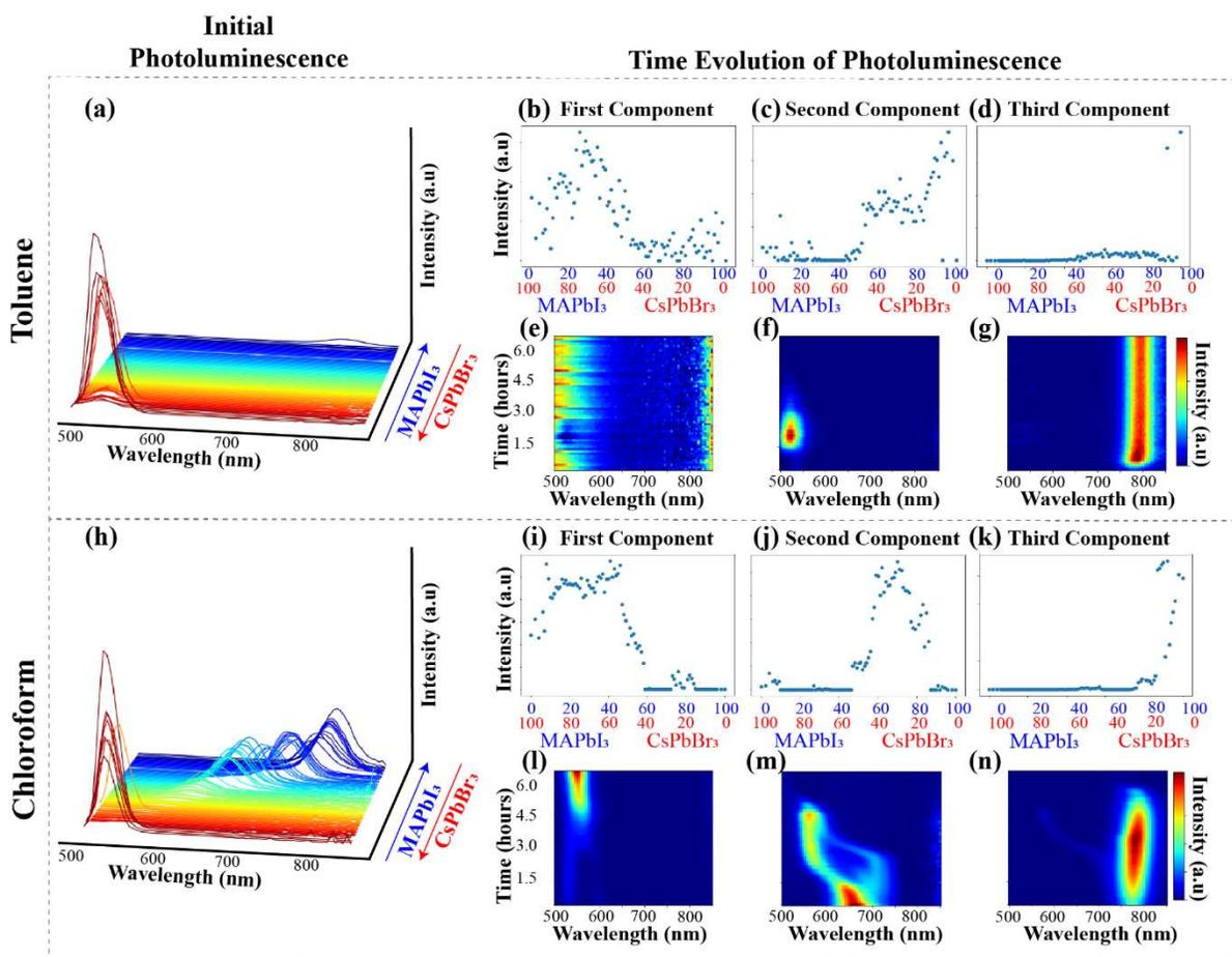
**Figure 4. Double cation and double halide system, MA<sub>x</sub>Cs<sub>1-x</sub>Pb(I<sub>x</sub>Br<sub>1-x</sub>)<sub>3</sub>.** a) initial PL behavior when toluene is used as the antisolvent. b), c), and d) are the loading maps for CsPbBr<sub>3</sub>-rich compositions, solution solutions of CsPbBr<sub>3</sub> and MAPbI<sub>3</sub>, and MAPbI<sub>3</sub>-rich compositions,
