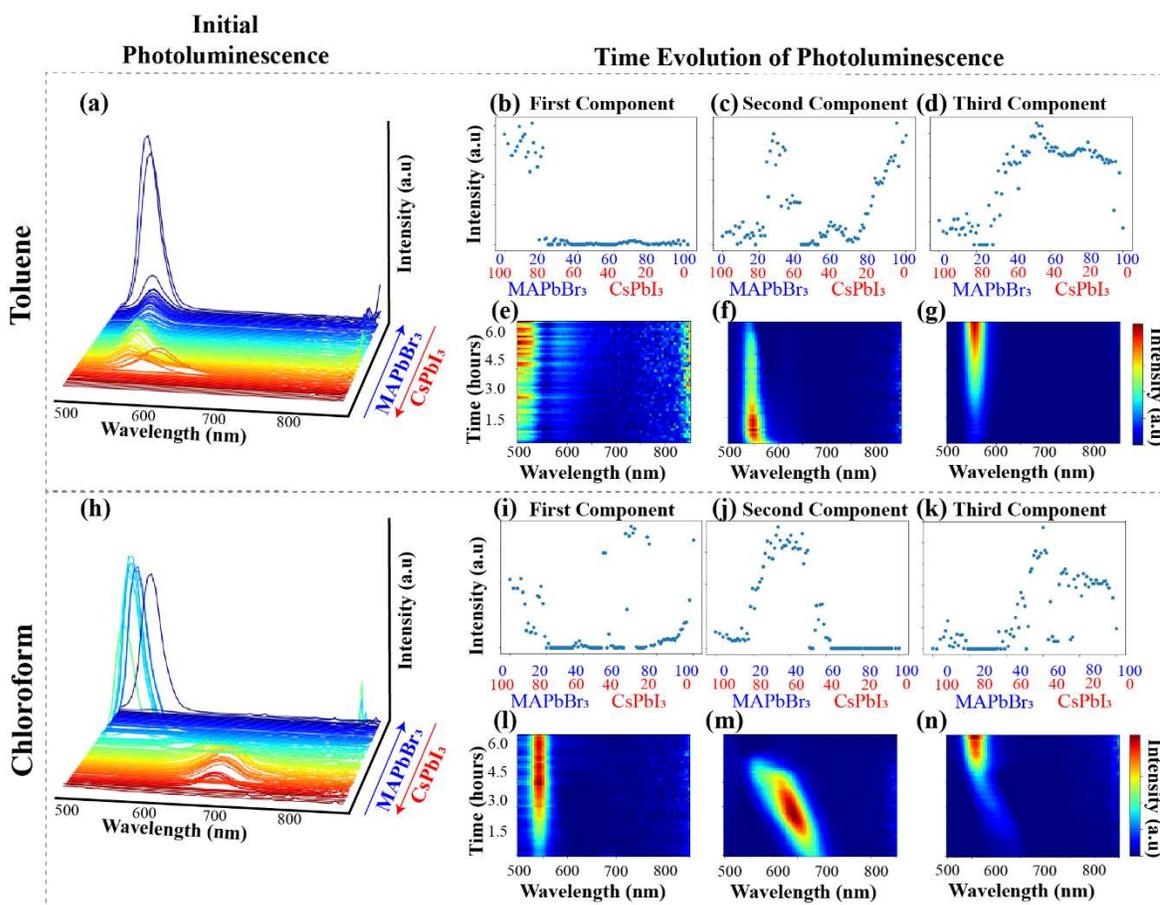
**Figure 5. Double cation and double halide system, MA<sub>x</sub>Cs<sub>1-x</sub>Pb(Br<sub>x</sub>I<sub>1-x</sub>)<sub>3</sub>.** **a)** initial PL behavior when toluene is used as the antisolvent. **b), c), and d)** are the loading maps for CsPbI<sub>3</sub>-rich compositions, solution solutions of CsPbI<sub>3</sub> and MAPbBr<sub>3</sub>, and MAPbBr<sub>3</sub>-rich compositions,
