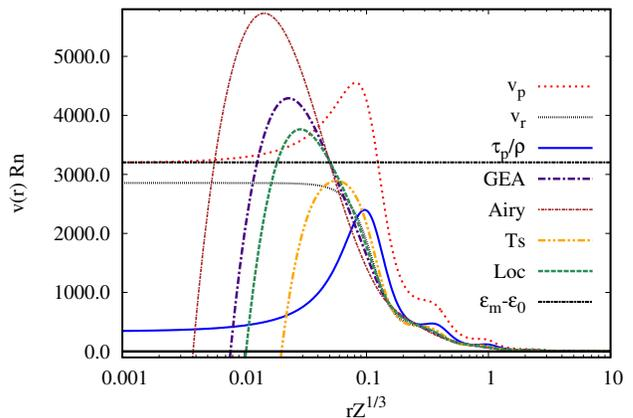
FIG. 3. Components of the Pauli potential,  $\frac{\tau_p}{\rho(r)}$ ,  $v_p$ , and  $v_r$ , for Rn, compared to response potential from several DFT models. GEA is the gradient expansion approximation [Eq. (19)], Airy, the Airy gas gradient expansion [Eq. (22)], loc, the fit to the local KED for high- $Z$  atoms [Eq. (23)], Ts, the Tsirelson model [Eq. (24)].  $\epsilon_M - \epsilon_0$  is difference between highest and lowest occupied eigenvalues.
