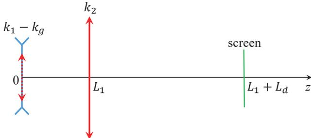
FIG. 3. A simplified model of the overlapped rf and solenoid fields in solenoid scan beamline.
