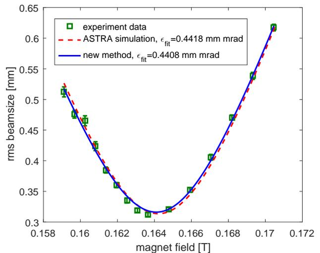
FIG. 5. green squares: experiment data of the beam spot sizes versus the solenoid strength in the PITZ beamline. Red dashed line: fitting curve based on the *Method Two*. Blue solid line: fitting curve based on the new method.
