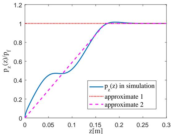
FIG. 4. blue line:  $p_z(z)/p_f$  simulated in ASTRA using the axial rf field profile; red dots: approximation 1 of  $p_z(z)$ ,  $p_z(z) = p_f$ ; magenta dashed line: approximation 2 of  $p_z(z)$  (see Eqn. 32).
