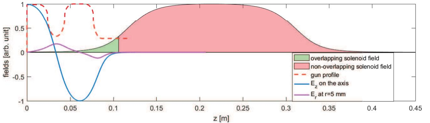
FIG. 2. Field distributions of the THU photoinjector. The dashed red line exhibits the gun profile. The blue line indicates the longitudinal electric field on the axis and the magenta line indicates the radial electric field at an off-axis position  $r=5$  mm. The light green area indicates that the axial solenoid field overlaps with the rf field, and the light red area indicates that the field that doesn't overlap with the rf field.
