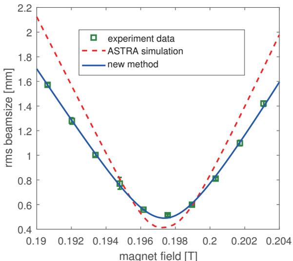
FIG. 6. green squares: experiment data of the beam spot sizes versus the solenoid strength in the AWA beamline. Blue solid line: fitting curve based on the new method. Red dashed line: simulated results in ASTRA using the thermal emittance fitted with the new method.
