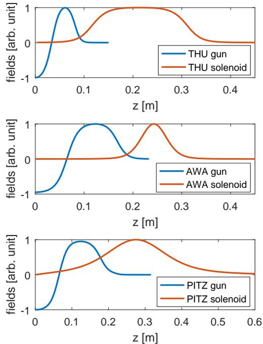
FIG. 1. rf and solenoid field profiles of the THU, AWA and PITZ photoinjectors. The blue lines indicate the rf field and the red lines indicate the solenoid field. Both the rf and the solenoid field profiles are normalized by the respective peak magnitude.
