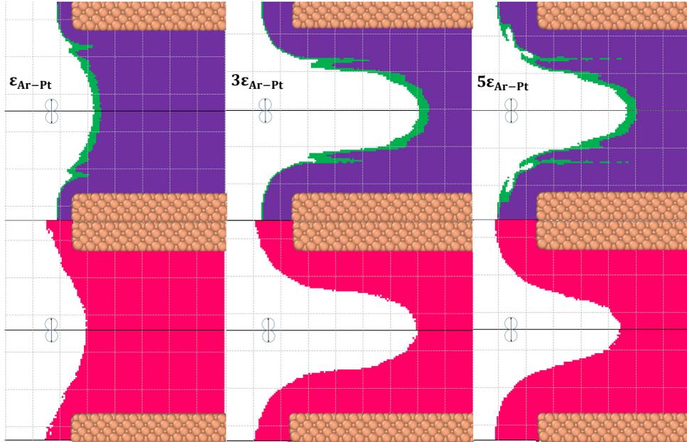
Figure 4: The effect of interface detection methods with different wall-fluid interaction potential strength. Tests were performed on M2 using 8 nW H/C. Top row: Density-based interface definition. Green and purple colors represent the liquid phases obtained using the density cutoff values of 250 and 350 kg/m<sup>3</sup>, respectively. Bottom row: Liquid phase obtained using energy-based interface detection method.
