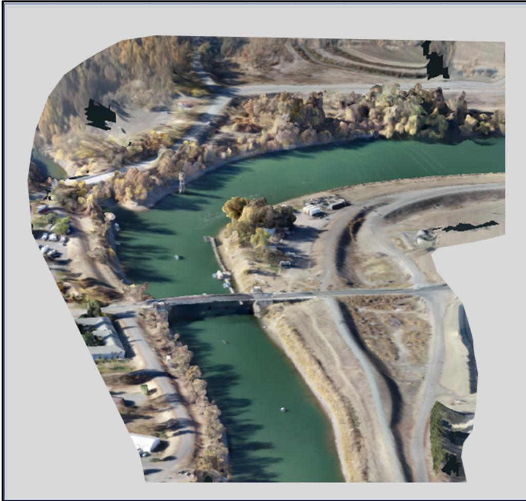
**Figure 5.** Textured model showing the measured above water topographic data, derived from aerial photography using SfM for Sacramento River at Knights Landing. Flow is from the top right to the bottom.
