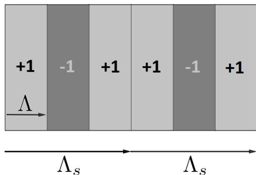
FIG. 7: An example  $\chi^{(2)}$  Moiré grating with a Moiré period that is three times the length of the poling period. The effect of the Moiré period is to create a single double-length poling period after each Moiré period.
