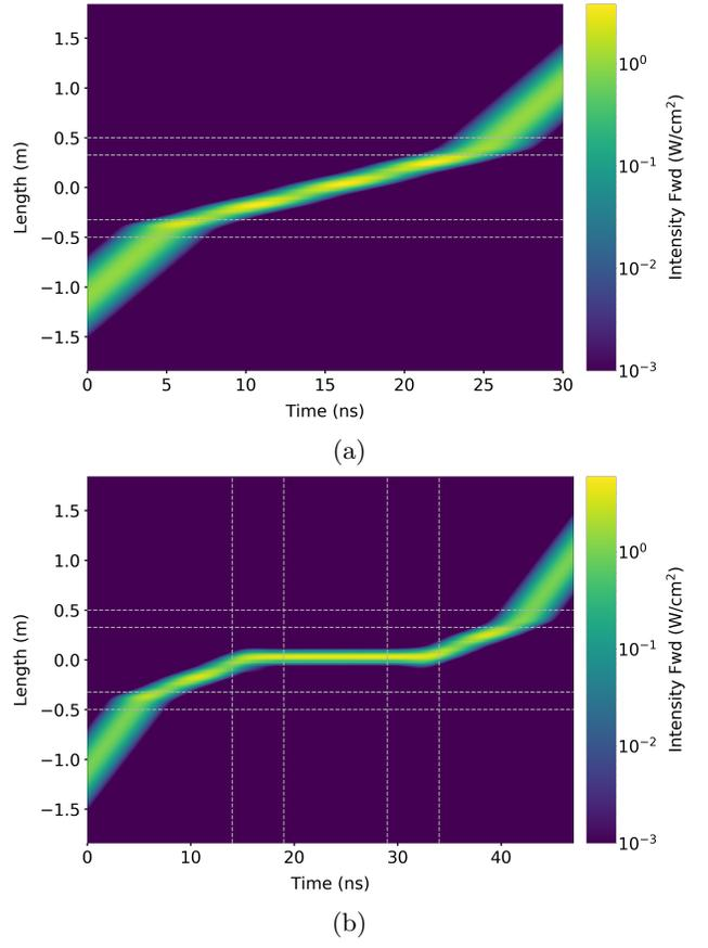
FIG. 4: Intensity distribution in space and time of a pulse propagating through (a) a static Moiré grating and (b) a dynamic Moiré grating with  $\mu = 2$ . The grating has a raised cosine apodization with 65% flat top with parameters  $L = 1\text{m}$ ,  $\Lambda_S = 4\text{mm}$ ,  $\lambda_B = 1.55\mu\text{m}$ ,  $\bar{n} = 1.445$ ,  $\delta n = 10^{-3}$ . The pulse has FWHM spectral bandwidth of 320MHz with carrier wavelength  $\lambda_B$ .
