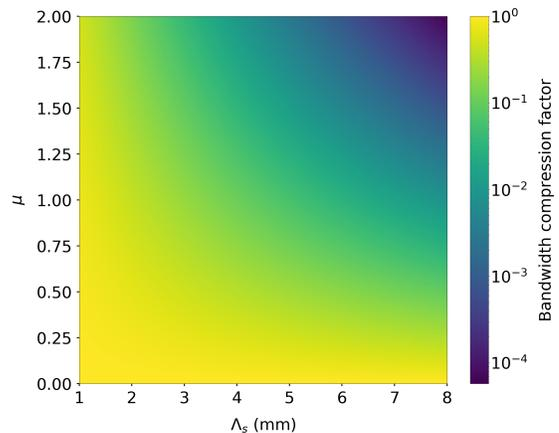
FIG. 6: Bandwidth compression factor depending on  $\Lambda_S$  and  $\mu$  in a dynamic Moiré grating with parameters  $L = 20\text{cm}$ ,  $\lambda_B = 1.55\mu\text{m}$ ,  $\bar{n} = 1.445$ ,  $\delta n = 10^{-3}$ .
