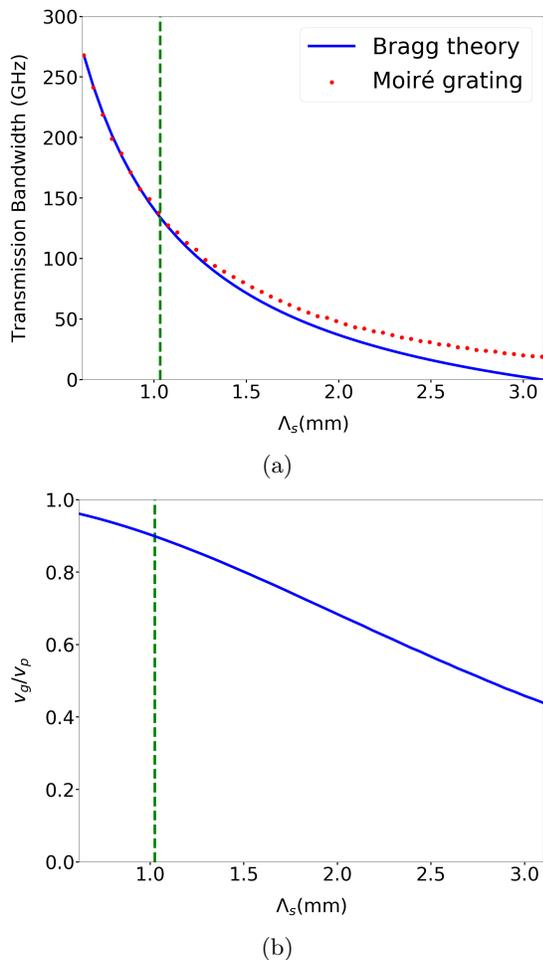
FIG. 2: (a) Moiré transmission bandwidth calculated from Bragg theory and a numerical calculation, and (b) group velocity of a Moiré grating versus Moiré period  $\Lambda_S$ . The grating has a Gaussian apodization with parameters  $L = 20$  cm,  $\lambda_B = 1.55\mu\text{m}$ ,  $\bar{n} = 1.445$ ,  $\delta n = 10^{-3}$ . The vertical green line indicates the Moiré period beyond which the approximation of the Moiré grating by two Bragg gratings begins to break down.
