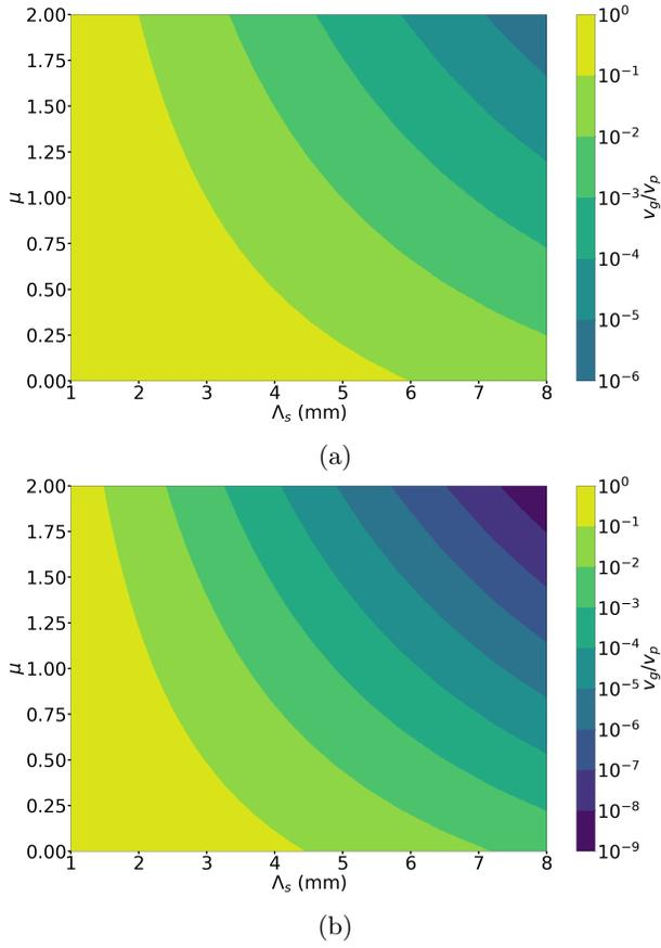
FIG. 3: Group velocity of (a) a Moiré grating and (b) a  $\pi$  phase-shifted grating versus  $\Lambda_s$  and  $\mu$ . The grating has a raised cosine apodization with 70% flat top with parameters  $L = 20\text{cm}$ ,  $\lambda_B = 1.55\mu\text{m}$ ,  $\bar{n} = 1.445$ ,  $\delta n = 10^{-3}$ .
