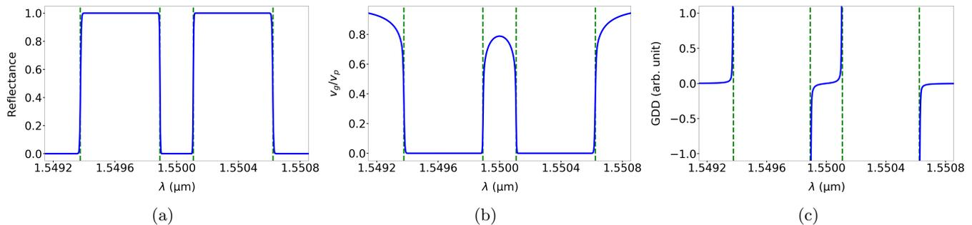
FIG. 1: (a) Reflection spectrum, (b) group velocity and (c) group delay dispersion for a Gaussian apodized Moiré grating with parameters  $\bar{n} = 1.445$ ,  $\delta n = 10^{-3}$ ,  $\lambda_B = 1550$  nm,  $\Lambda_s = 2.68$  mm and  $L = 10$  cm.
