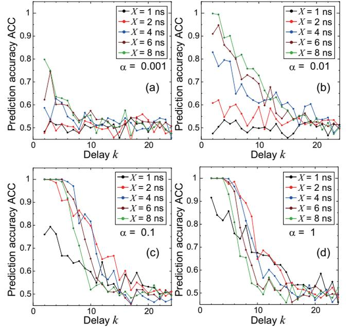
FIG. 12. Prediction accuracy ACC plotted against delay  $k$ , which were estimated by solving XOR problems using 72-dimensional  $\mathbf{y}(n)$  with  $d_k(n) = \text{XOR}(u(n-1), u(n-k))$  for delay  $k = 2, \dots, 24$ :  $\alpha =$  (a) 0.001, (b) 0.01, (c) 0.1, and (d) 1, where black, red, blue, brown, and green dots represent the results for  $X = 1, 2, 4, 6,$  and  $8$  ns, respectively, and colored lines connecting nearest-neighbor dots are guides.
