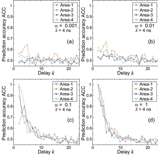
FIG. 13. Prediction accuracy ACC plotted against delay  $k$ , which were estimated by solving XOR problems using 18-dimensional  $\mathbf{y}(n)$  with  $d_k(n) = \text{XOR}(u(n-1), u(n-k))$  for delay  $k = 2, \dots, 24$ :  $\alpha =$  (a) 0.001, (b) 0.01, (c) 0.1, and (d) 1, where grey, orange, pale-blue, and pale-green dots represent the results with  $X = 4$  ns for Area-1, -2, -3, and -4, respectively, and colored lines connecting nearest-neighbor dots are guides.
