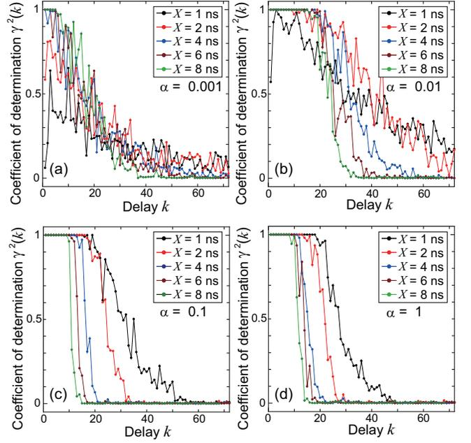
FIG. 14. Coefficient of determination  $\gamma^2(k)$  plotted against delay  $k$ , which were estimated by solving delay tasks using 72-dimensional  $\mathbf{y}(n)$  with the target output  $d(n) = u(n-k)$  for delay  $k = 1, \dots, 72$ :  $\alpha =$  (a) 0.001, (b) 0.01, (c) 0.1, and (d) 1, where black, red, blue, brown, and green dots represent the results for  $X = 1, 2, 4, 6,$  and  $8$  ns, respectively, and colored lines connecting nearest-neighbor dots are guides.
