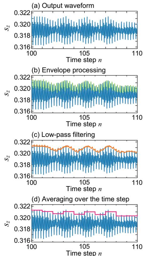
FIG. 10. Post processing of a reservoir output signal, which is executed in the order of (a) reservoir output signal, (b) an envelope processing, (c) a low-pass filtering, and (d) averaging over the time step  $X$ . Blue lines in (a)–(d) are the same signal obtained at Detector 1 when  $\alpha = 0.1$  and  $X = 4$  ns. Colored lines in (b)–(d) are the signals after the processing. The  $x_i(n)$  value in (d) is assigned to  $y_i(n)$  ( $i = 1, \dots, 72$ ) in  $\mathbf{y}(n)$ .
