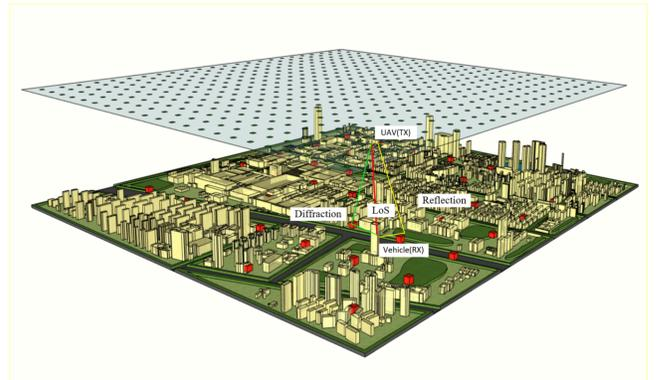
Fig. 2. Acquisition of massive RT-based data.
