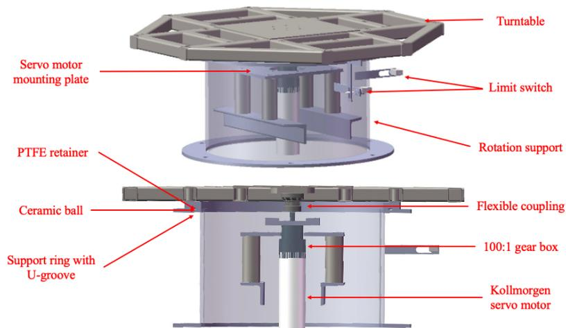
**Figure 4.** Drawings of the turntable.
