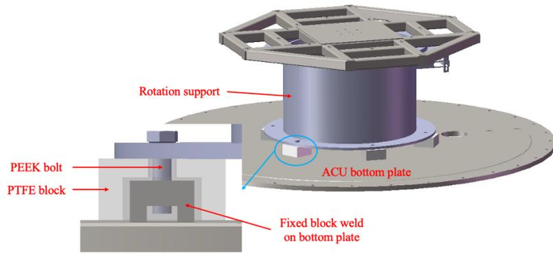
**Figure 15.** The ACU electronics insulation plan.
