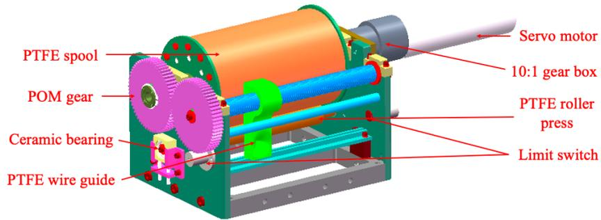
**Figure 5.** Drawing of the radioactive source spool.
