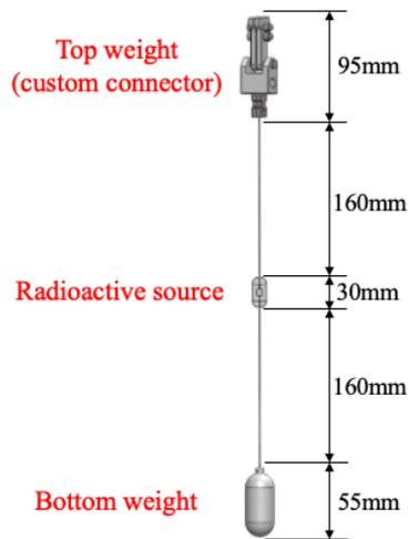
**Figure 6.** A schematic diagram of a radioactive source assembly. A custom connector serves as a top weight. The  $6 \times 6 \text{ mm}^2$  SS radioactive source capsule is enclosed in a PTFE enclosure. A Nickel block enclosed by a PTFE enclosure serves as the bottom weight.
