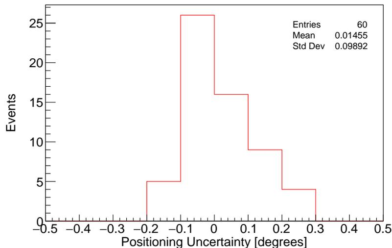
**Figure 19.** The measured angular uncertainty of the turntable.
