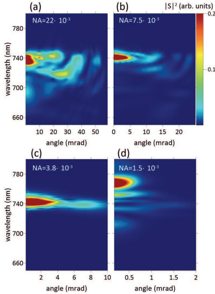
Fig. 4. Numerically simulated frequency-angular distribution of optical intensity  $|S|^2$  for the laser pulse with initial energy  $E = 1$  mJ under various focusing conditions.
