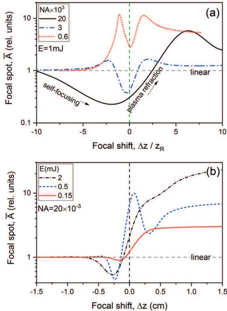
Fig. 7. Relative laser beam focal waist area  $\bar{A}$  versus propagation distance at different (a) numerical apertures  $NA$  and (b) pulse energy  $E$ .
