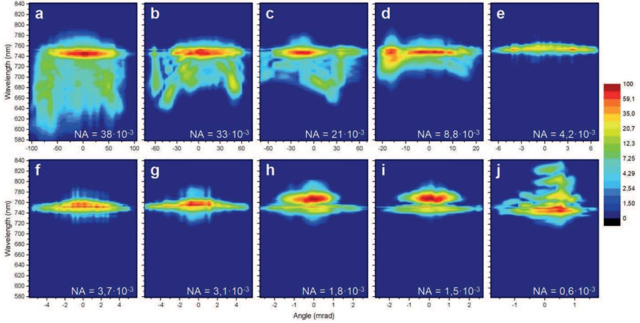
Рис.2. (a-j) Experimental frequency-angular spectra of the femtosecond pulse ( $E = 1$  mJ) at different numerical apertures  $NA$ . The laser beam spatial diameter  $D_0$  is 3 mm except for (b), (f) and (i), where  $D_0$  is 8 mm.
