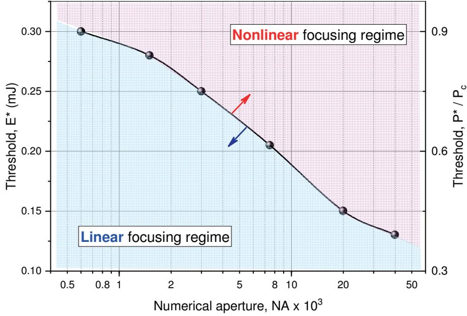
Fig.6. Threshold energy  $E^*$  and threshold peak power  $P^*$  of the laser pulse linear focusing at different numerical apertures  $NA$ .
