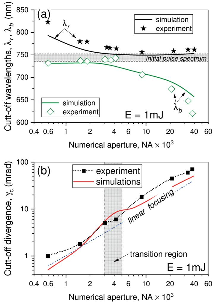
Fig. 3. (a) Maximum  $\lambda_r$  (circles) and minimum  $\lambda_b$  (squares) cut-off wavelengths of the laser pulse spectrum and (b) cut-off spatial angle  $\gamma_c$  after the filamentation in air as a function of a numerical aperture  $NA$ . The initial laser pulse spectrum and linear focusing transition region are marked by shaded areas.
